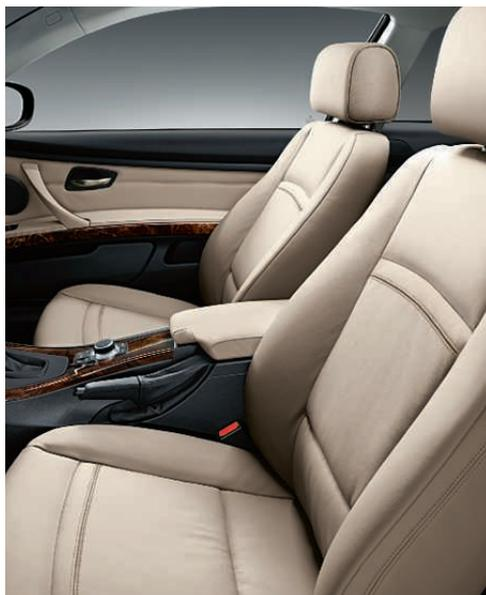
**8-way adjustable front seats** in the 328i and 328i xDrive are eight-way adjustable for the driver and six-way adjustable for the front passenger. Both seats also include a two-way headrest. The driver's seat provides individual adjustments for seat height and backrest, fore and aft position and seat angle.
