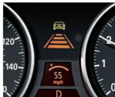
**Active Cruise Control (ACC) with Stop & Go**<sup>3</sup> allows the driver to preset both a desired speed and distance. When ACC recognizes slower vehicles ahead, it reduces your speed to maintain the preset distance. Stop & Go can bring you to a complete stop if traffic calls for it. When you press the accelerator, ACC resumes your speed according to your presets.
