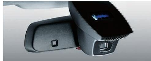
**Automatic high beams** let you enjoy the convenience of switching between high and low beams automatically. When the Automatic high beams system is activated, an image sensor at the back of the rear-view mirror monitors oncoming traffic and lighting conditions. Based on this data, the system decides whether or not the high beams should be switched on. When it detects vehicles ahead, or the sensor dictates that ambient light is sufficient, the high beams are automatically switched off.
