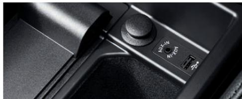
**Auxiliary input port** lets you connect an external audio source, such as an iPod® or MP3 player.
