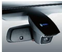
When activated, **Automatic high beams** switch high-beam headlights to low beams automatically when there is oncoming traffic or another car just ahead, or when the road is sufficiently illuminated. Then when the sensor detects decreased illumination, the low beams are automatically switched back to high beams.
