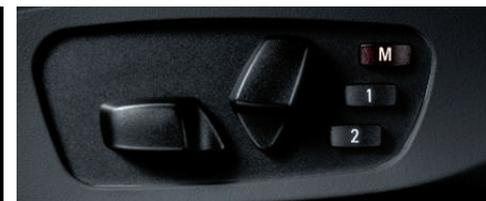
**Power seat adjustments** included with eight-way power front seats allow customized comfort and convenience for driver and front passenger. The two-setting memory system automatically adjusts the driver's seat and side-view mirror positions, with individual preferences available at your fingertips.
