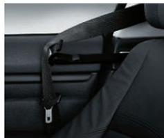
**Automatic safety-belt assistant** for the two front seats makes buckling up easier by bringing the belt forward whenever you get into the vehicle. As soon as the safety belt is clicked, the arm retracts into its housing. (If the safety belt for an occupied seat isn't used, the arm retracts after one minute or as soon as the vehicle reaches a speed of about 4 mph.)
