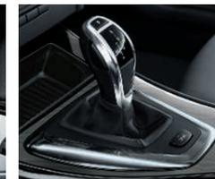
**7-speed Double Clutch Transmission (DCT)** provides smooth, lightning-quick gear changes and enhanced fuel efficiency by automatically shifting between two transmission structures. While one gear is disengaging, the next is already in position. Shift gears manually without a clutch by using paddle shifters or the gear selector.
