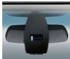
**Rain sensor** uses infrared light to measure the amount of falling rain and spray from other vehicles. When there is oncoming traffic or another car just ahead, or when the road is sufficiently illuminated, the rain sensor automatically adjusts the windshield wiper interval as needed. **Automatic headlight control** activates headlights by means of a sensor that responds to darkness.
