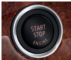
**Engine Start/Stop button**<sup>1</sup> and key fob control the engine. Upon inserting the key fob into the starter switch slot, and the electronic identification system confirming that it is the correct key fob, the engine can be started (or later, shut off) by pressing the Start/Stop button.
