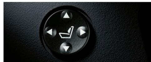
**Lumbar support** for front seats adds four-way adjustable comfort for the lower back. The up/down and in/out lumbar support positioning is electrically adjustable.
