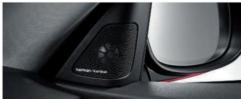
**Harman Kardon® Surround Sound Audio System** with vehicle-specific equalizing and powerful 420W amplifier. The 11-speaker system includes four tweeters, two midrange speakers located in the door panels and two midrange speakers located under the rear shelf space, two bass speakers located under the front seats and one midrange center channel speaker located in the dashboard.
