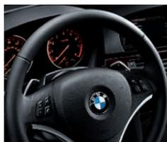
**Steering wheel-mounted paddle shifters** provide sportier manual gear shifts without the use of a clutch. When equipped with STEPTRONIC automatic transmission and the M Sport Package, paddle shifters are automatically added. Paddle shifters are included in the BMW 335is with the 7-speed Double Clutch Transmission.
