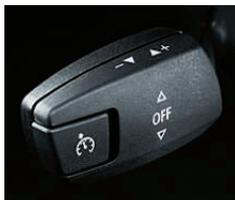
**Dynamic Cruise Control** lets you store and maintain a chosen speed above 20 mph. It is activated via the left-hand steering column switch, and deactivated by applying the brakes or via the switch.<sup>2</sup>
