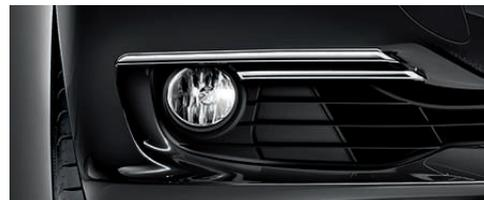
**Halogen free-form foglights**, built into the front air dam, enhance your margin of safety in bad visibility. Ellipsoid free-form technology provides for even light distribution on the road.
