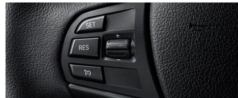
**Dynamic Cruise Control<sup>4</sup>** lets you set and keep to a chosen speed above 20 mph, including automatic application of the brakes when driving downhill. It is activated and regulated via controls positioned on the left side of the steering wheel, and deactivated by applying the brakes or switching off the feature.
