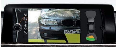
**Rear-view Camera** shows on the Control Display the area behind your vehicle. Working with Park Distance Control, interactive guidelines indicate if a parking space can accommodate the vehicle, and display parking trajectories and turn angles. The Rear-view Camera is activated by engaging reverse gear.
