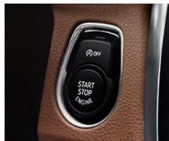
**Engine Start/Stop button and Comfort-go key** control the engine. After the electronic identification system recognizes and confirms the correct key code, you can start (or later, turn off) the engine by pressing the Start/Stop button. (Foot must be on the brake pedal in order to start.)
