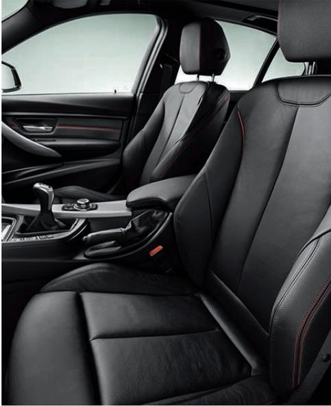
**Ten-way adjustable front sport seats** make the driving experience more enjoyable with adjustments for fore/aft, seat height, backrest angle, seat angle and thigh support. Side bolsters can be power-adjusted to comfortably fit your back while helping to hold you firmly in place during cornering. Includes two-way headrests with Active Head Restraints feature.
