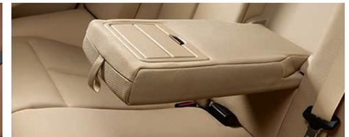
**Rear center armrest** includes two cupholders integrated into the front of the armrest. When not in use, they can be stored out of sight by sliding them back into the armrest. The armrest swings up to create a third rear passenger seat.
