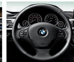
**Three-spoke leather-wrapped multi-function steering wheel** provides buttons on the left for operating the cruise control functions; buttons on the right adjust all audio-related functions, including Bluetooth enabled mobile phone (if so equipped), the wheel.
