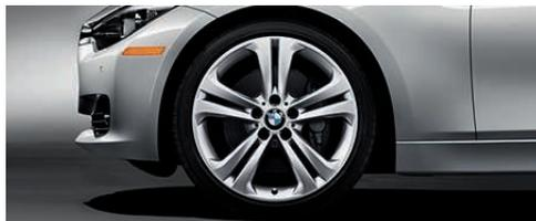
**Double Spoke (Style 401)** light alloy wheels and **run-flat<sup>1</sup> performance<sup>2</sup> tires<sup>3</sup>**. In front: 19 x 8.0 wheels and 225/40 tires; in back: 19 x 8.5 wheels and 255/35 tires.
