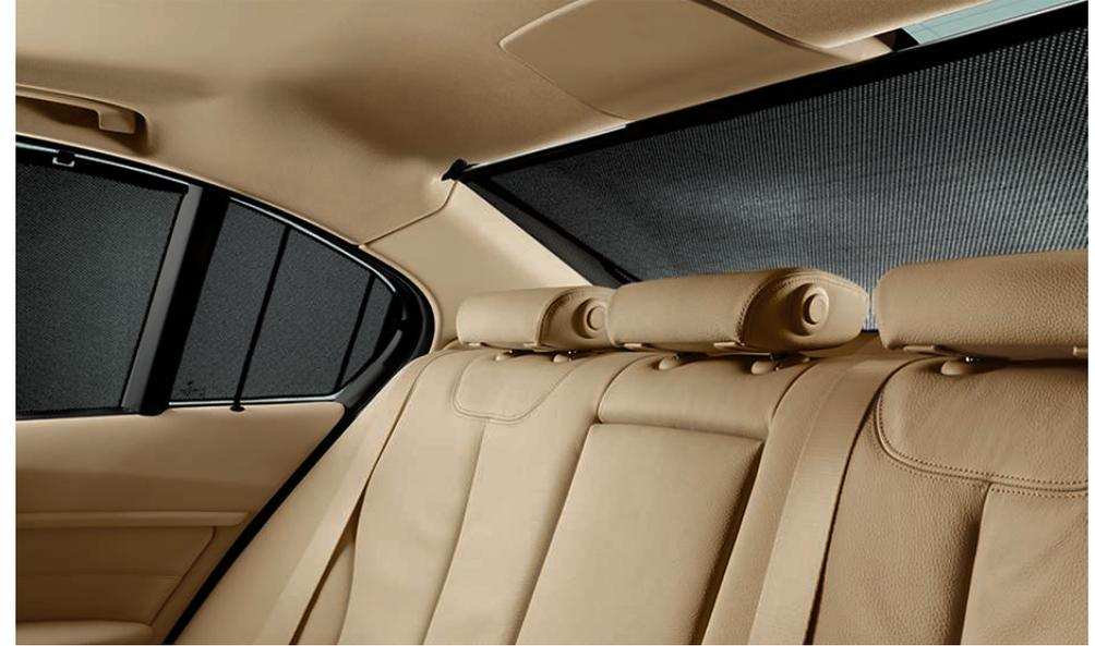
**Power sunshade for the rear window** can be raised and lowered at the press of a button. Together with manual sunshades for the rear side windows, this feature maintains occupant privacy, helps eliminate glare, and helps lower the cabin temperature by reflecting intense sunlight. (European model shown.)
