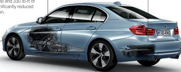
**High-performance lithium-ion battery:** this highly efficient battery supplies the BMW ActiveHybrid 3 with the power needed for electric-only driving for 2–2.5 miles at speeds of up to 37 mph. It also adds a temporary 55-hp boost to the gasoline engine for increased dynamic performance. Using a more advanced form of Brake Energy Regeneration, this storage unit is recharged whenever you lift your foot off the accelerator pedal.
