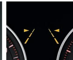
**Lane Departure Warning feature<sup>1</sup>** uses a camera to recognize when your vehicle is crossing over roadway lane markings or is changing lanes without signaling, and warns you by sending a mild vibration through the steering wheel. The system can be turned on and off via a button by the steering wheel.
