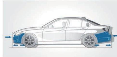
**Impact-absorbing bumpers** and compressible "crush tubes" front and rear help absorb the force of impact in collisions up to 9 mph, helping to minimize damage to the vehicle's body and simplifying repairs. Only at higher impact speeds do structural supports begin to deform, dissipating impact energy to help protect occupants.
