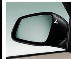
**Active Blind Spot Detection** warns if a vehicle is in your blind spot, or if a vehicle is approaching at high speed in the passing lane, by displaying a visual signal in the exterior mirror casing. The system also warns you by making the steering wheel vibrate should you then use the turn-signal indicator before executing a lane change.
