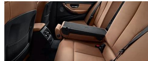
**Rear fold-down seats** allow flexible combinations of passengers and cargo. Use the folding 40-20-40 seats with through-loading feature for transporting skis or other long items.
