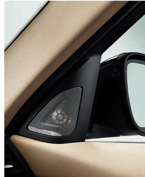
**Harman Kardon® Surround Sound System** is a 16-speaker, multi-channel system that outputs reproduction of the surround information contained in the stereo signal in a nine-channel format as well as 5.1 surround sound from a DVD source. Includes a powerful 600-watt digital amplifier with nine channels. The system compensates for driving noise in smooth steps with speed-dependent equalizing.
