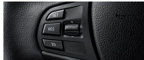
**Dynamic Cruise Control<sup>4</sup>** lets you set and keep to a chosen speed above 20 mph, including automatic application of the brakes when driving downhill. It is activated and regulated via controls positioned on the left side of the steering wheel, and deactivated by applying the brakes or switching off the feature.
