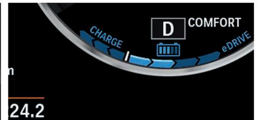
**All-electric driving:** the 40 kW (55 hp) output of the electric motor allows all-electric driving over longer distances. Using Driving Dynamics Control to activate the ECO PRO mode, the transmission uncouples the engine and shuts it off when you take your foot off the accelerator. This feature enables the BMW ActiveHybrid 3 to "sail" downhill almost silently up to 100 mph. When the ECO PRO mode is deactivated, it is possible to sail at speeds of up to 50 mph.
