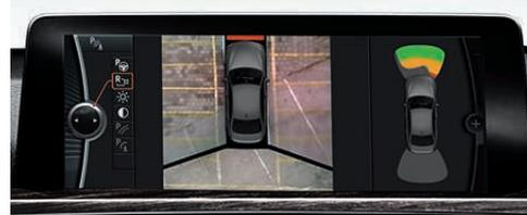
**Surround View** displays video images of approaching traffic on the Control Display. Side-view Cameras positioned in the front bumpers show traffic approaching the front of the vehicle from the sides, such as when exiting a garage. The Top-view Camera provides video images of the road alongside the doors, taken by cameras positioned in the exterior mirrors.
