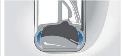
**Run-flat tires.** Thanks to reinforced sidewalls, run-flat tires maintain their shape and rim position even after suffering a complete loss of tire pressure. They allow you to continue driving at a reduced speed until you reach a safe area to change a tire or wait for Roadside Assistance. The Tire Pressure Monitor alerts you when there is a drop in tire pressure; if the loss is severe, an acoustic warning is triggered.
