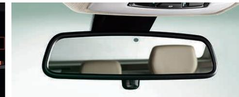
**Automatic-dimming interior and exterior mirrors** sense the bright headlights of vehicles behind you and automatically darken. The exterior power-adjustable side-view mirrors include fold-in function. **BMW Universal garage-door opener** takes the place of up to three remote-control devices. It can activate remote functions outside the vehicle, such as garage-door openers or home-lighting systems.
