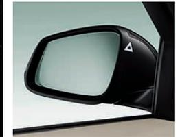
**Active Blind Spot Detection** warns if a vehicle is in your blind spot, or if a vehicle is approaching at high speed in the passing lane, by displaying a visual signal in the exterior mirror casing. The system also warns you by making the steering wheel vibrate should you then use the turn-signal indicator before executing a lane change.
