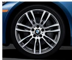
**Double Spoke (Style 403M)** light alloy wheels and **run-flat<sup>1</sup> performance<sup>2</sup> tires<sup>3</sup>**. In front: 19 x 8.0 wheels and 225/40 tires; in back: 19 x 8.5 wheels and 255/35 tires.
