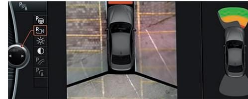
**Park Distance Control (PDC)** uses ultrasonic sensors in the front and rear bumpers to help you judge the distance to other cars and unseen objects when parking. The beeping becomes faster as your bumper approaches the object, turning into a constant tone when the distance is less than 12 inches.
