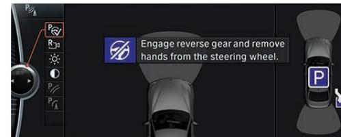
**Parking Assistant** makes parking a breeze. Using ultrasonic sensors integrated into the side indicators, the system searches for and measures parking spaces. When a space at least four feet longer than your vehicle is spotted, it is shown on your Control Display. Shift into reverse and the system takes control of steering your vehicle into the space.
