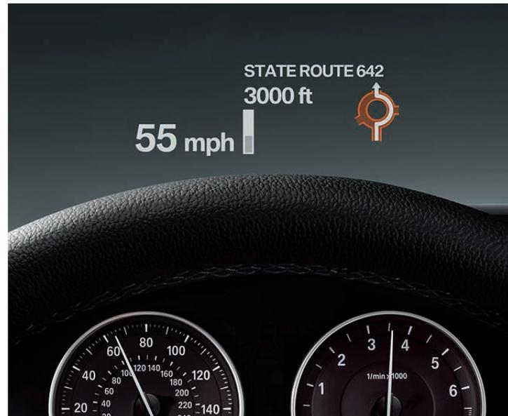
**Head-up Display** projects important travel information, such as vehicle speed and Check Control warnings, onto the windshield directly in your field of vision. Data is shown in full color, making information even more precise and easier to process. Additional information, including Lane Departure Warning messages and Navigation directional arrows and instructions, can also be displayed.
