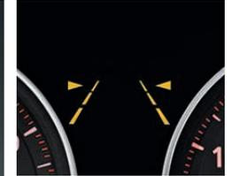
**Lane Departure Warning feature<sup>1</sup>** uses a camera to recognize when your vehicle is crossing over roadway lane markings or is changing lanes without signaling, and warns you by sending a mild vibration through the steering wheel. The system can be turned on and off via a button by the steering wheel.
