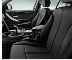
**Eight-way adjustable front seats** offer manual adjustment fore/aft, backrest angle, seat height and two-way headrests with Active Head Restraints feature.
