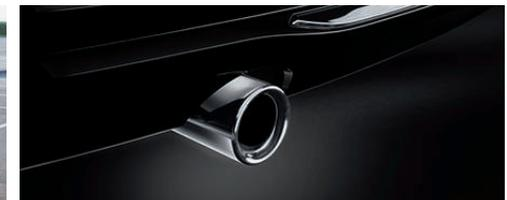
**Exhaust tailpipe** configuration identifies the all-new 3 Series Sedans. There are two on the left side of the 326i; on the 335i, there is one tailpipe on the left and one on the right.
