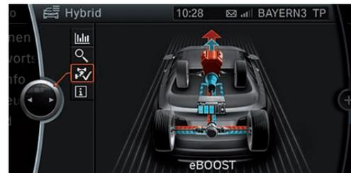
**Boost function:** when required, energy from the high-performance battery is used to enable a short-term boost of power. A benefit of this technology is strong and immediate power delivery.
