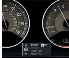
**Driving Dynamics Control with ECO PRO mode** lets you change the driving character of the 3 Series Sedan with just the push of a button. The switch customizes accelerator response characteristics, power steering characteristics and Dynamic Stability Control (DSC) thresholds. Choose between ECO PRO, COMFORT, SPORT and SPORT+ modes; each activates different settings for extra sporty, more relaxed or maximized fuel-efficient driving modes.
