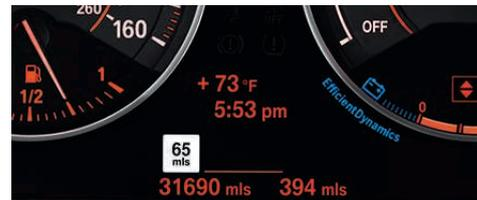
**Speed Limit Information** detects local speed limit signs and shows them in the Info Display or Head-up Display, if so equipped.
