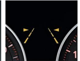
**Lane Departure Warning<sup>1</sup>** uses a camera to recognize when your vehicle is crossing over roadway lane markings or is changing lanes without signaling, and warns you by sending a mild vibration through the steering wheel. The system can be turned on and off via a button by the steering wheel.
