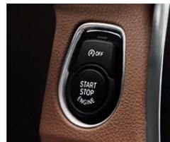
**Engine Start/Stop button** control the engine. After the electronic identification system recognizes and confirms the correct key code, you can start (or later, turn off) the engine by pressing the Start/Stop button. (Foot must be on the brake pedal in order to start.)
