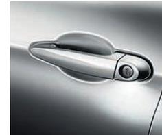
**Comfort Access system** offers convenient keyless access to your vehicle. Carrying the remote key in a pocket or purse allows you to unlock the doors by touching the door handle. The hands-free trunk-lid opening function automatically unlocks and opens the trunk when you stand behind the vehicle and move your foot under the center of the rear bumper.
