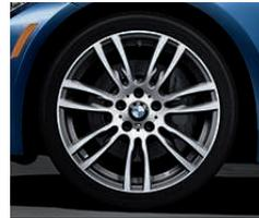
**Star Spoke (Style 403M)** light alloy wheels and **run-flat<sup>1</sup> performance tires.<sup>2</sup>** In front: 19 x 8.0 wheels and 225/40 tires; in back: 19 x 8.5 wheels and 255/35 tires.
