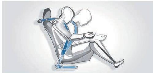
**BMW restraint system** for the driver and front passenger combines three-point safety belts, automatic safety-belt pretensioners, seat bolsters that help prevent occupants from sliding forward, and Active Head Restraints. This system helps provide optimum restraint in a collision.
