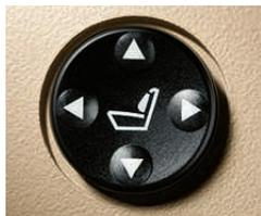
**Lumbar support** for front seats adds four-way adjustable comfort for the lower back. Lumbar support can be adjusted up/down and in/out.
