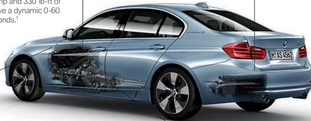
**High-performance lithium-ion battery:** this highly efficient battery supplies the BMW ActiveHybrid 3 with the power needed for electric-only driving for up to 2.5 miles at speeds of up to 47 mph in ECO PRO mode. It also adds a temporary 55-hp boost to the gasoline engine for even greater dynamic performance. Using an advanced form of Brake Energy Regeneration, this storage unit is recharged whenever you lift your foot off the accelerator pedal.
