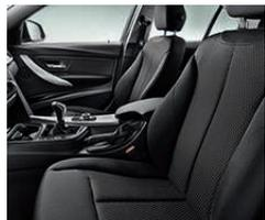
**10-way adjustable front seats** offer manual adjustment fore/aft, backrest angle, seat angle, seat height and two-way headrests with Active Head Restraints feature.
