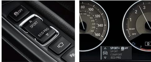
**Driving Dynamics Control with ECO PRO mode** lets you change the driving character of the 3 Series Sedan with just the push of a button. The switch customizes accelerator response characteristics, power steering characteristics and Dynamic Stability Control (DSC) thresholds. Choose between ECO PRO, COMFORT, SPORT and SPORT+ modes; each activates different settings for extra sporty, more relaxed or maximized fuel-efficient driving modes.
