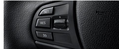
**Dynamic Cruise Control<sup>3</sup>** lets you set and keep to a chosen speed above 20 mph, including automatic application of the brakes when driving downhill. It is activated and regulated via controls positioned on the left side of the steering wheel, and deactivated by applying the brakes or switching off the feature.
