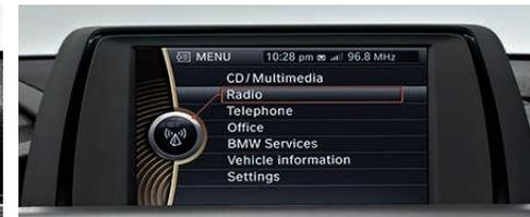
**BMW anti-theft AM/FM stereo CD/MP3 audio system** offers Radio Data System (RDS), Auto-Store, and 3-channel FM diversity antenna system. Song titles are displayed on the 6.5-inch color monitor (shown), or on the 8.8-inch color monitor included in the BMW ActiveHybrid 3 or in vehicles equipped with the Navigation system.
