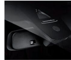
**Rain sensor** uses infrared light to measure the amount of rain. When the wipers are in the "intermittent" mode, the rain sensor automatically adjusts the windshield-wiping interval as needed.
