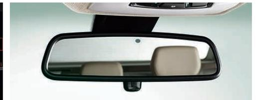
**Automatic-dimming interior and exterior mirrors** sense the bright headlights of vehicles behind you and automatically darken. The exterior power-adjustable side-view mirrors include fold-in function.
