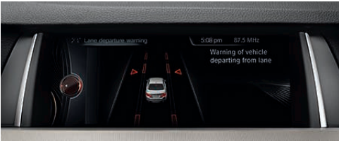
Driver Assistance Plus Package increases your active safety quotient in all types of traffic situations, with Active Blind Spot Detection, Side- and Top-view Cameras, and Speed Limit Info. It also includes the full collection of Active Driving Assistant features: Lane Departure Warning, Frontal Collision Warning, Pedestrian Warning, and City Collision Mitigation.
