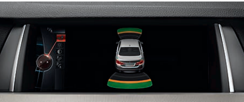
Rear-view Camera shows on the Control Display the area behind your vehicle. Guidelines indicate if your vehicle can fit in a parking space, and display parking turn angles. The Rear-view Camera is activated by engaging reverse gear. Park Distance Control (PDC) helps you judge distance to other vehicles and unseen objects when parking. The warning beeps come faster as the bumper approaches the object, turning into a constant tone at less than 12 inches. Side- and Top-view Cameras display video images of traffic approaching the front of the vehicle from the sides, such as when exiting a garage or parking space. The Top-view Camera provides birdseye video images of the road alongside the doors, taken by cameras positioned in the exterior mirrors.
