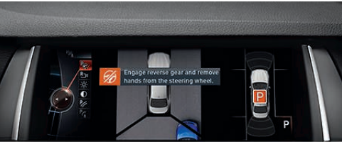
Parking Assistant makes parking a breeze by searching for suitable parking spots and then steering your vehicle into them. Simply press the "Park Assistant" button, then drive along potential parking spaces on the left or right side of the road, staying below 22 mph and no more than five feet away. Using ultrasonic sensors integrated into the side indicators, the system searches for and measures parking spaces. When a space at least four feet longer than your vehicle is spotted, it is shown on your Control Display. Shift into reverse and Park Assistant takes control of steering your vehicle into the selected space; you operate the accelerator and brake pedals. The acoustic and visual warnings of Park Distance Control (PDC) provide assistance.
