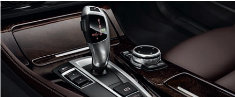
8-speed STEPTRONIC automatic transmission with Adaptive Transmission Control (ATC) provides extremely fast synchronized shifting in either the Sport or Manual shift mode. By increasing the number of gears to eight, the transmission provides a more efficient shifting sequence; thanks to the new coasting function, it also offers improved fuel economy.
