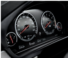
The extended instrument cluster features Black Panel Display with permanently illuminated white surrounds for speedometer and rev counter plus fuel level and oil temperature displays.
