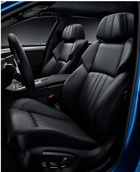
M Multi-contour seats for driver and front passenger. In addition to M seat adjustments, includes power upper backrest angle, backrest width and thigh support; comfort headrests with power height adjustment; lumbar support and memory function for driver and front passenger.
