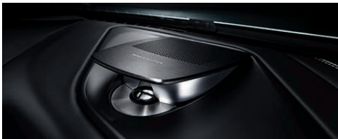
Bang & Olufsen® High-End Surround Sound System offers innovative Dirac Dimensions™ signal processing and 16 speakers with a total output of 1200 watts, including a retractable center speaker. Acoustic Lens Technology ensures consistent sound quality at all seats. Choose between two sound settings: "Studio" for particularly crisp sound, and for a more open sound space, "Expanded."
