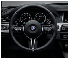
Multi-function M leather steering wheel with gear shift paddles and two M Drive buttons. The double-spoke design and stainless steel M logo add to its sporting good looks.
