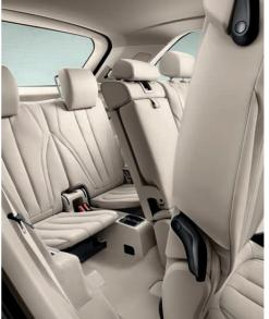
Third-row seating allows greater flexibility in transporting up to seven people. In addition to the two fold-down seats with inertia-reel safety belts, a center console includes two cupholders, and there is heating for the third-row footwells. The second row of seats can be folded down using the Easy Entry Function; there is also a grip plate by the C-pillar. When not in use, each third-row seat can be lowered individually into the floor for increased cargo space.
