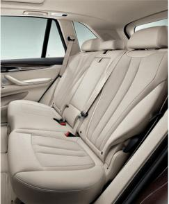
fore and aft, providing greater legroom or increasing the cargo space, as needed.
