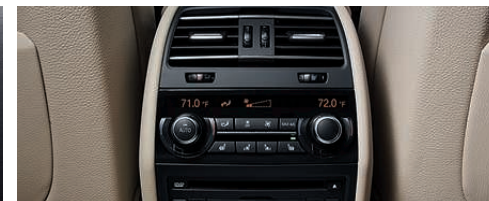
Four-zone automatic air conditioning delivers draft-free ventilation. In front, automatic climate control includes fully separate left/right controls, solar sensor, automatic recirculation, and heat-at-rest feature. The rear cabin offers left/right temperature-controlled outlets and auto ventilation.
