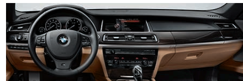
Three-spoke leather-wrapped multi-function M sport steering wheel features reduced diameter, special thumb rests and shift paddles.
