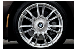
V Spoke (Style 301 I) 20 x 8.5 front, 20 x 10.0 rear light alloy wheels with 245/40 front, 275/35 rear run-flat 1 performance tires. 2
