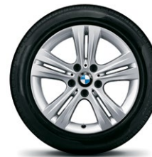
Double Spoke light alloy wheels (Style 392), 17 x 7.5; and 225/50 run-flat 1 all-season tires 2
