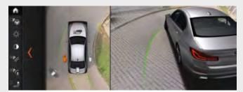
☐ Parking Assistant Plus makes parking and manoeuvring the vehicle easier. It features Surround-view including Top-view, Remote 3D view, Panorama view, PDC and Park Assist with linear guidance, which parks the vehicle parallel or perpendicular to the lane completely automatically. The system works by measuring potential spaces while driving past at a low speed.
