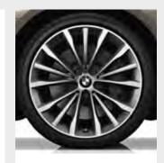
$\hfill \square$  19" light alloy W-spoke style 663 wheels Bicolour, front 8J x 19 with 245/40 R19 tyres and rear 9J x 19 with 275/35 R19 tyres.
