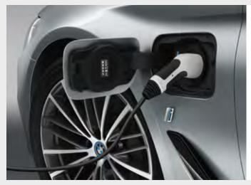
The charging port for the external charging of the high voltage battery can be found behind a flap on the vehicle's front side panel on the left. The charging port is protected from harmful environmental effects by a special gasket ring.
