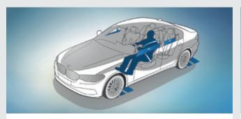
☐ **Dynamic Safety** is the BMW ConnectedDrive preventive passenger protection system. Dynamic Safety warns the driver if it detects signs of tiredness, safety belts are pre-tensioned in critical situations, electric seats are returned to upright positions and the windows and sliding roof are closed. After an accident occurs, the brakes are automatically applied until the car reaches a standstill.
