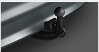
$\hfill\square$  The Towbar with electrically adjustable tow ball is approved for heavy loads of up to 2,000kg. In order to stabilise things, trailer stability control automatically brakes the pulling vehicle if the trailer begins to swing. The electronically adjustable tow ball is not visible when stowed under the rear apron.
