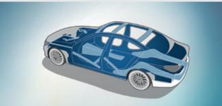
■ The extremely torsionally stiff but light **body construction** provides the basis for sporty driving dynamics, high-precision steering and agility. Additionally, it offers the passengers the best possible all-round protection.
