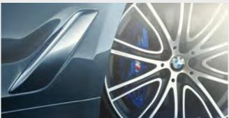
$\hfill \square$  The 20" BMW Individual light alloy V-spoke style 759 I wheels with M Sport braking system features exceptional braking performance. (M Sport braking system is not available on 520i/520d/520d xDrive models.)
