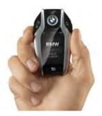
☐ The BMW display key shows various information about the vehicle's status and allows selected functions to be controlled with an integrated touch display.
