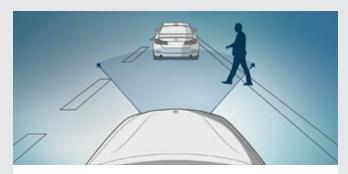
■ Person warning with city braking function actively assists the driver with the prevention of collisions involving pedestrians. It is active at speeds of up to 35mph and preconditions the brakes for increased responsiveness. In the event of an emergency, the system prevents a collision or ensures that the collision speed is considerably reduced.2
