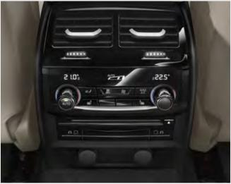
☐ Automatic air conditioning with four-zone control comes with the equipment included in automatic air conditioning with two-zone control with extended features, along with two air vents in the B columns. Additionally, the rear passengers can individually adjust their own climate via a separate control element with display.
