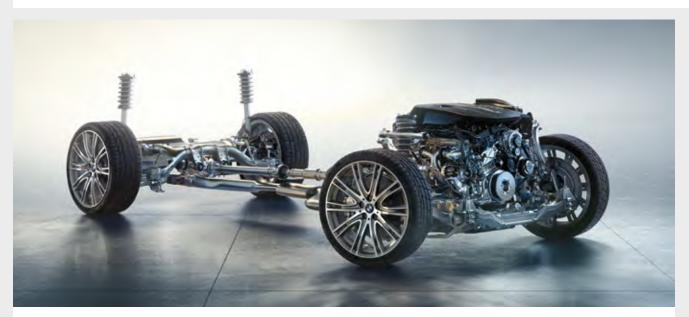
**Integral Active Steering** combines support that varies based on the steering angle on the front axle, and rear wheels that also contribute to steering. At lower speeds, it offers greater manoeuvrability and agility by turning the rear wheels opposite the front wheels. Beginning around 37mph, the rear wheels turn parallel to the front wheels, to increase stability and comfort.<sup>1</sup>
