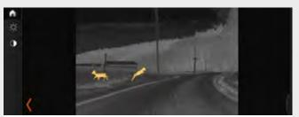
☐ BMW Night Vision with pedestrian recognition makes people and large animals visible on the Control Display from a distance using infrared imaging and illuminates them with the Dynamic Light Spot in the main headlight. An additional warning system is also automatically activated when the vehicle is started, regardless of the status of the imaging display.
