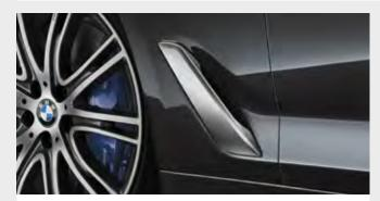
■ The Air Breathers channel air to the front wheels, reducing air resistance, fuel consumption and  $CO_2$  emissions.
