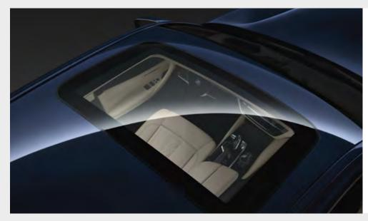
☐ The electric glass sunroof with slide and lift function, including an electric sliding interior roof, anti-trap protection, as well as comfort opening and closing, allows the airflow to be individually regulated to create a pleasant interior climate. The integrated wind deflector prevents draughts from developing in the interior and ensures a lower level of wind noise.
