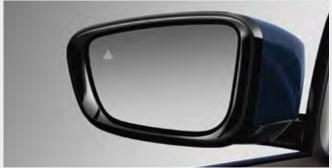
☐ If the indicator is on, the radar-based Lane Change Warning² warns the driver of approaching vehicles in the blind spot as well as vehicles in the neighbouring lane. The system functions beginning at speeds of 6mph, and in dangerous situations, it causes the steering wheel to vibrate and the triangle symbol in the exterior mirror to blink.
