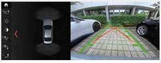
☐ The reversing assist camera enables improved orientation when reversing at speeds below 10mph, for example when parking. It shows the area behind the car on the Control Display. Interactive track lines for measuring distance and turning circles assist the driver when manoeuvring, obstacles are marked in colour.
