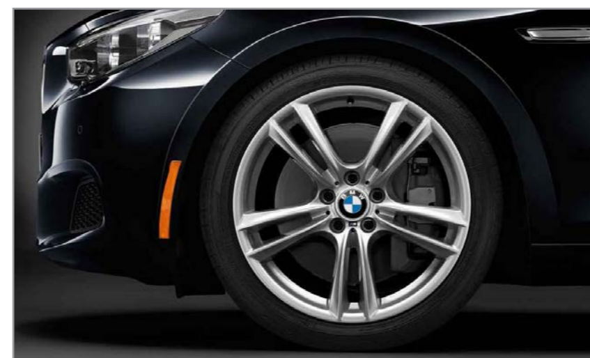
Double-spoke light alloy wheels (Style 303M) 20 x 8.5 front, 20 x 10.0 rear; and 245/40 front and rear 275/35 run-flat performance tires 1,2
