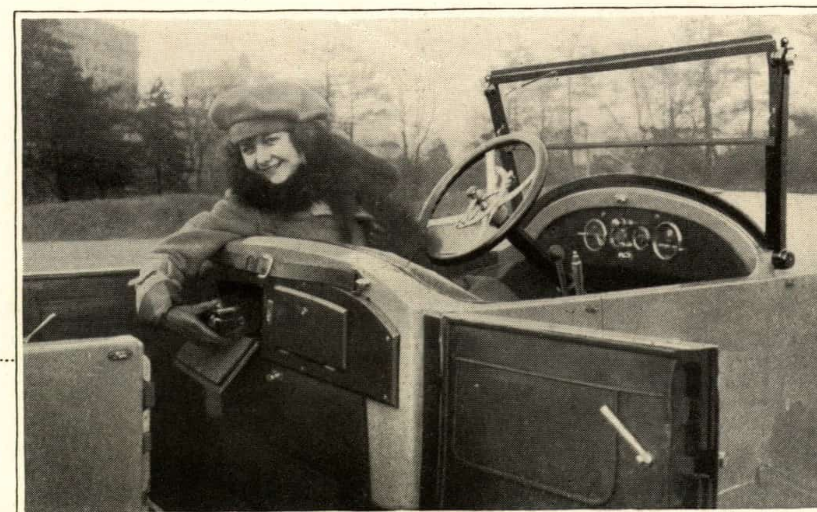
Tools, though rarely needed, are, nevertheless, conveniently at hand, being carried in the lock-fitted pocket of the left fore door
