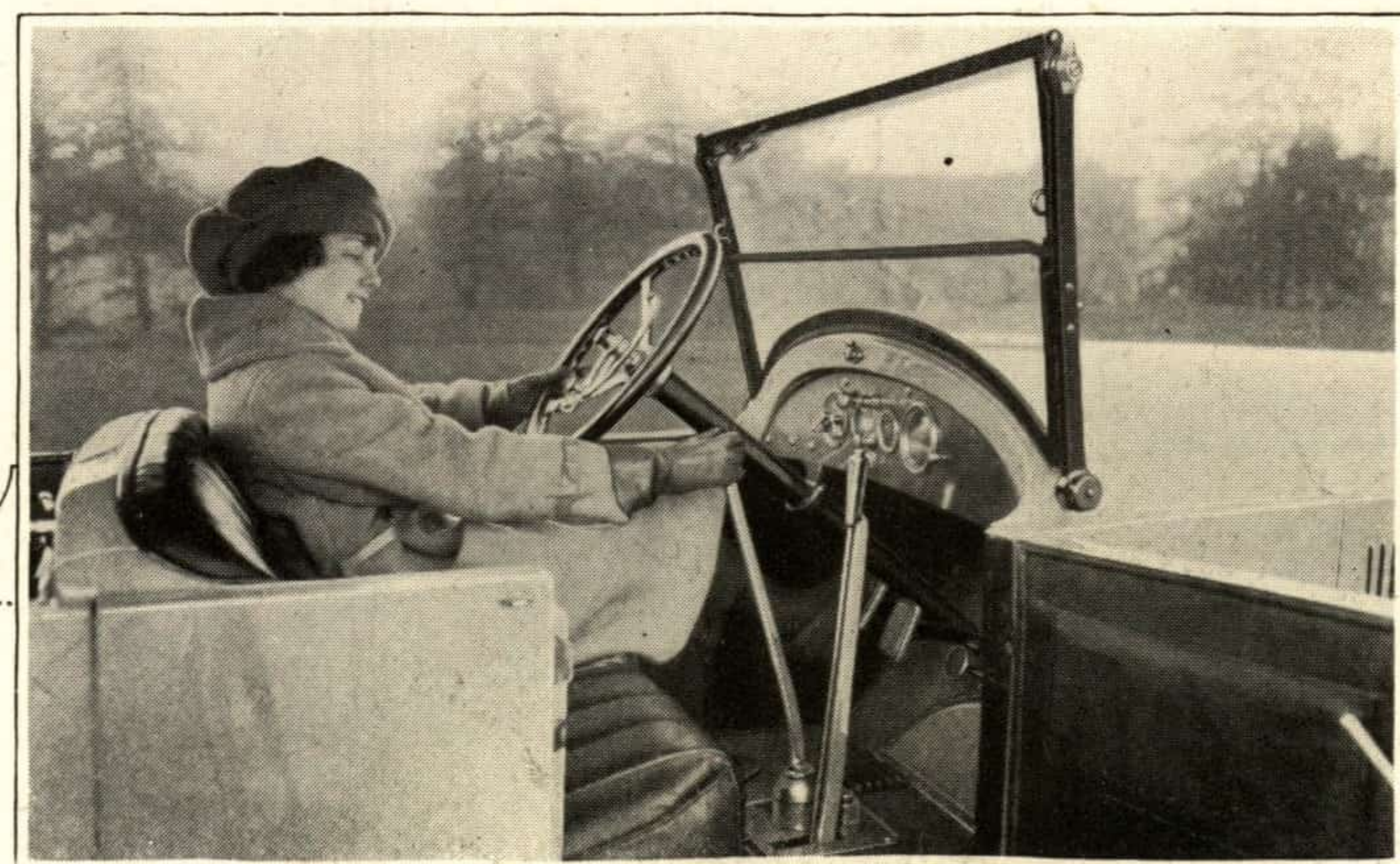
A small crank on the dash opens the hooded ventilator on the cowl, flooding the driving compartment with a current of fresh air
