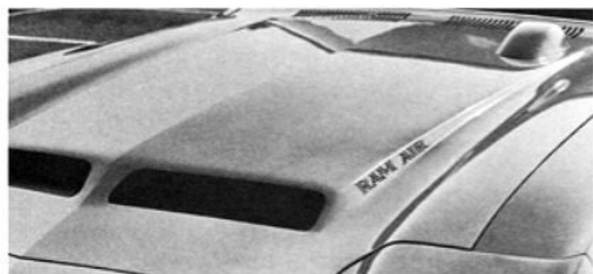
Ram Air Hood Inlet (Code 601—UPC WU3). Available on Formula and GTO with 455 H.O. 4-bbl. High-
