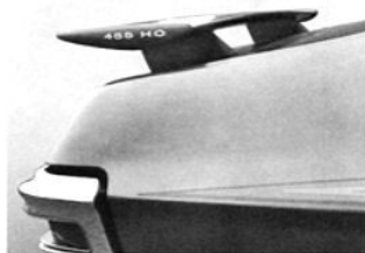
Rear Deck Airfoil (Code 604—UPC WT7). A real "spoiler" that helps keep downward pressure on rear of car. Flat back. Included in "The Judge" option. Available on T-37 and LeMans Hardtop Coupes, LeMans Sport and GTO. (D)
