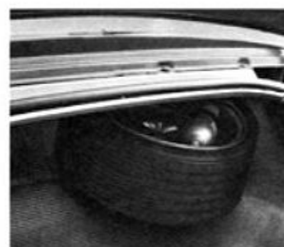
"Space-Saver Spare" Tire (Code 684—UPC N65) Adds approximately 3 cubic feet of usable luggage capacity. Easily inflated with handy pressure can and provides many miles of spare tire driving. (F) "Space-Saver Spare" Tire Inflators Replacements available from dealer. (D) See "Instant-Aire" Pump—this page.
