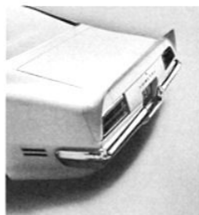
Rear Air Spoiler (Code 572—UPC D80). Sporty looking, body color, 3-piece rear deck attachment. Available for Formula, factory-installed. Available for Firebird, Esprit and Formula. (D)
