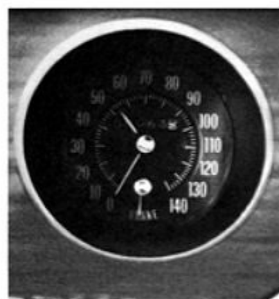
Safeguard Speedometer (Code 712—UPC U15). You set speed limit you desire with control knob. Buzzer signals if car exceeds this predetermined speed. Not available with Rally Gauge Clusters. Available T-37, LeMans, LeMans Sport, GTO and Grand Prix models. (F)
