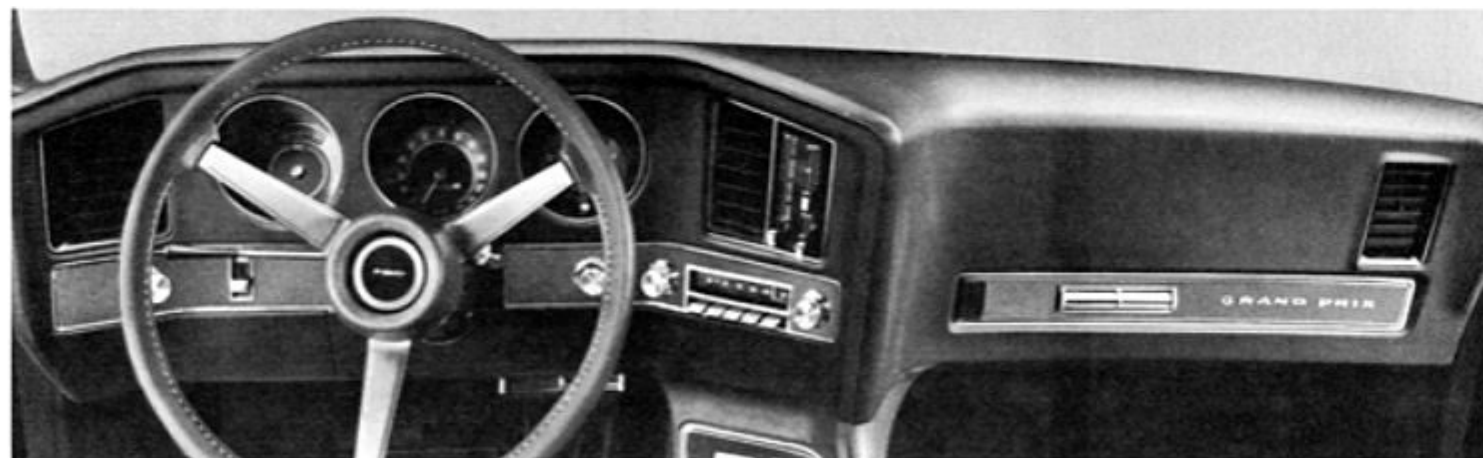
INSTRUMENT PANEL FOR GRAND PRIX WITH AUTOMATIC TEMPERATURE CONTROL.
