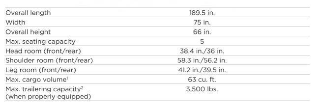
1 With rear seat folded. Cargo capacity limited by weight and distribution. 2 Before you buy a vehicle or use it for trailering section of the Owner's Manual. The weight of passengers, cargo and options or accessories may reduce the amount you can tow.
