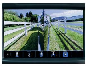
**Rear Side View** Provides a line of sight down each side of the truck and trailer to provide added views.
