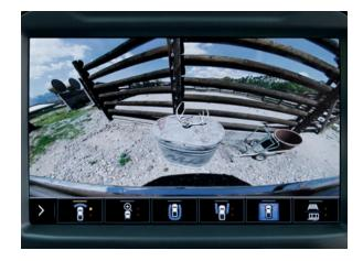
**Front Camera View** Displays front view with available guidelines to assist with parking and tight maneuvers.
