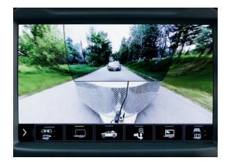
**Transparent Trailer** Allows the driver to virtually "see through" a conventional hitched box or camping trailer.
