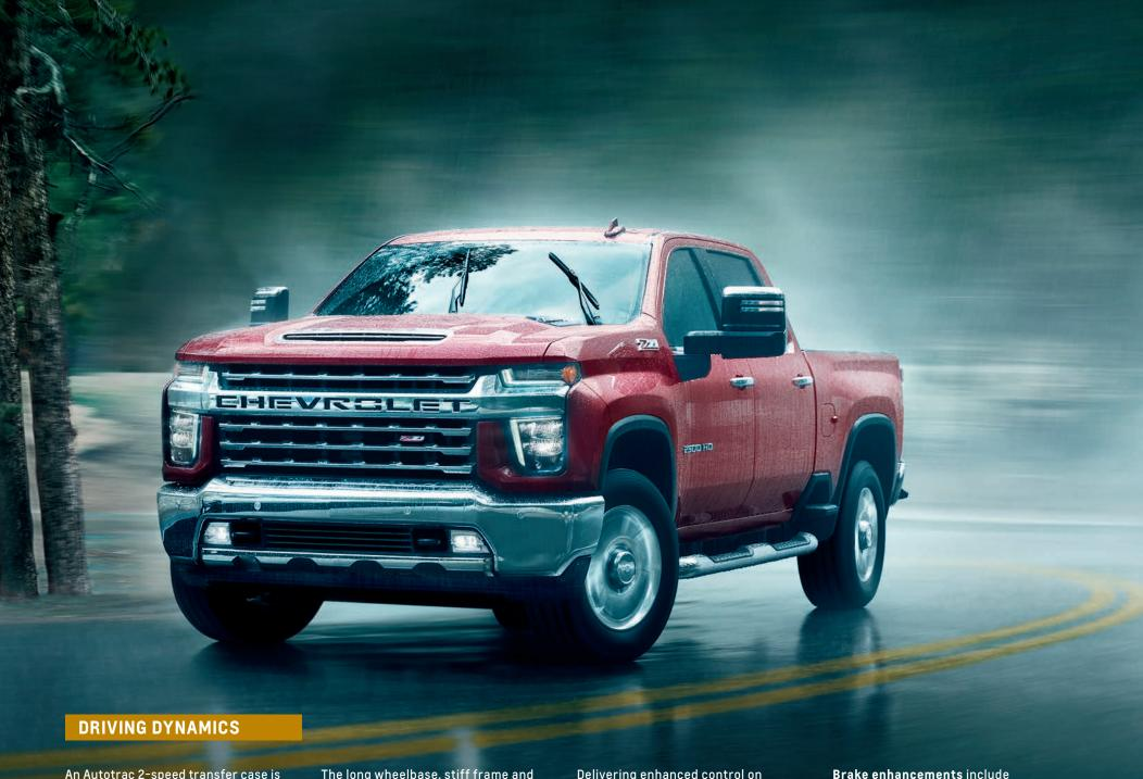
An Autotrac 2-speed transfer case is available and offers four drive modes: 2 High, 4 High, 4 Low and 4 Auto mode that automatically adjusts power sent to the front and rear axles for improved traction.
