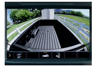
**Bed View** Allows you to see inside the cargo bed to help with fifth-wheel or gooseneck hitching and to check on cargo.
