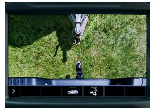
**Hitch View** Provides a close-up view of the receiver hitch to help with alignment when connecting to a trailer.
