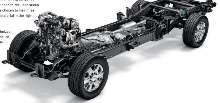
The chassis is 20% stiffer than the previous generation. To achieve that target, we used a combination of high-strength and ultra-high-strength steel throughout the cab and frame.
