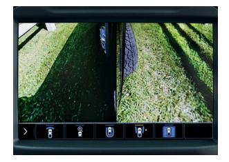
**Front Side View** Shows the position of the front tires when parking and during tight maneuvers.
