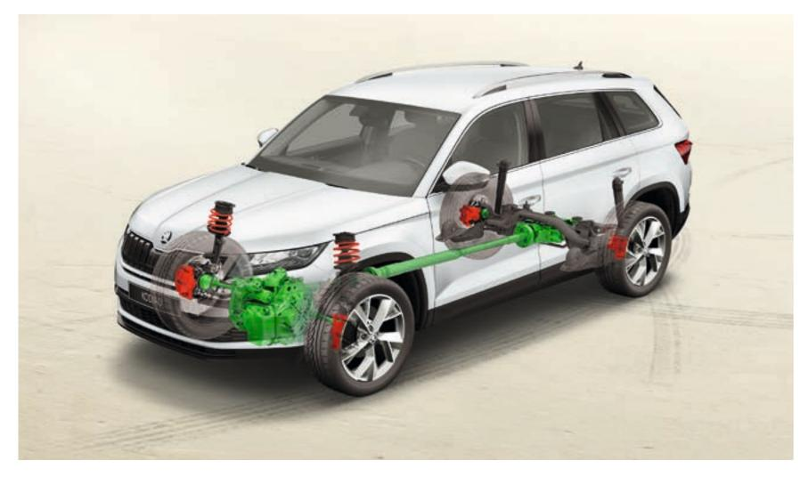
The 4x4 drive is provided by an inter-axle electronically-controlled multi-plate clutch. The coupling of the rear axle is automatic, so under normal conditions the car can utilise the advantages of frontwheel drive, and under extreme conditions the excellent traction of the 4x4 drive.
