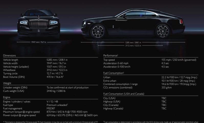
\* The engine is designed for Octane grade 95 fuel; however, it may be run on fuel with a minimum Octane grade of 91
