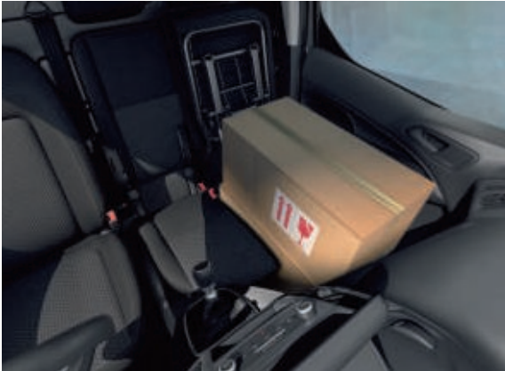
Flexible passenger's seat The centre seat folds flat and has a lift-up cushion and underseat storage. The outer seat base folds cinema-style so tall items may be carried. (Option on Van)
