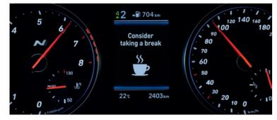
Driver Attention Alert (DAA): This standard feature raises safety and convenience to an entirely new level by continuously monitoring and analysing driving patterns. When a pattern of fatique or distraction is identified. DAA gets the driver's attention with an audible alert and pop-up message suggesting a break.
