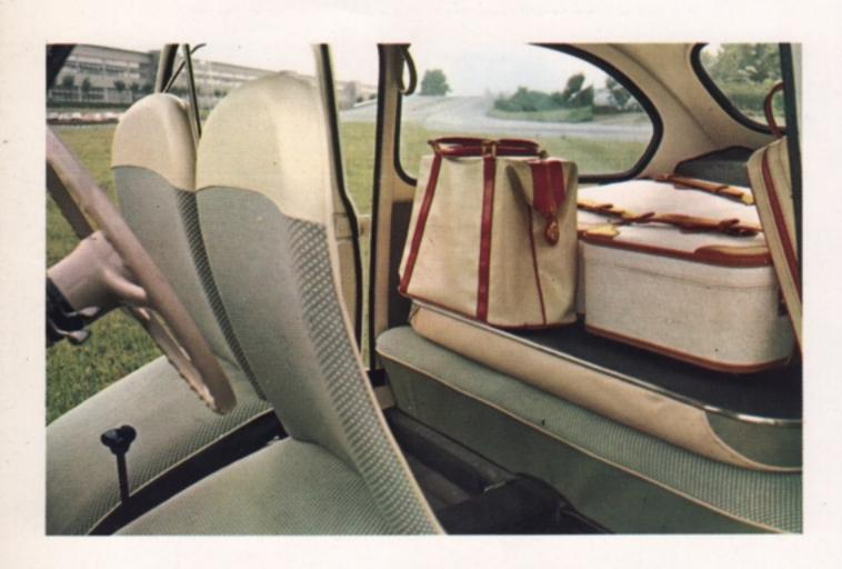
Well-lighted interior to seat four adults comfortably. Back of rear seat folds down to provide added luggage area when needed.
