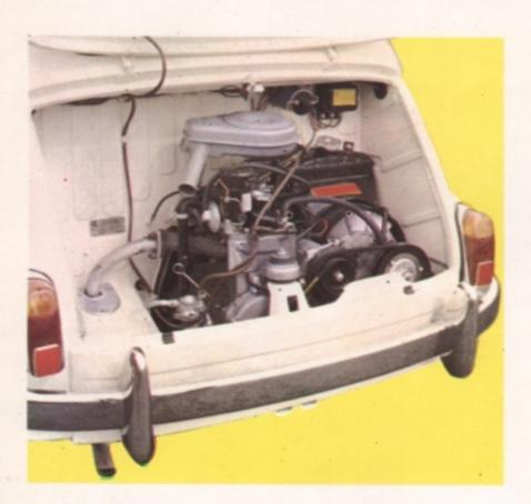
Engine, clutch, bevel-drive, differential and transmission all packed in a single unit easily accessible, located at the rear end of the Fiat 600D for better weight balance. The excellent road holding provided by the 4-wheel independent suspension is further improved by the added weight on the rear of the car. The O.H.V. engine is water cooled.
