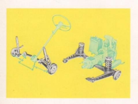
The 4-wheel independent suspension insures maximum road holding. On the front suspension a transverse leaf spring acting as a stabilizer is connected to the frame at two points by rubber mountings. The rear suspension is by swing arms with coil springs, and telescopic hydraulic shock absorbers.
