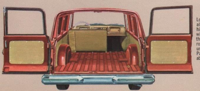
Loading the all new 'Jeep' Panel Delivery is no chore at all. Its big double rear doors swing all the way open to a high and wide 39½ in. by 55 in., the full inside height and width of the vehicle. Bed height is a short 23½ in. from the ground. There's a full 107 cu. ft. of usable cargo space—room to accommodate bulky loads of up to 1200 lbs. Yet unlike many competitors, when fully loaded, the 'Jeep' Panel Delivery still handles with ease, rides with unbelievable smoothness.
