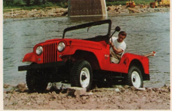
'Jeep' 4-wheel drive puts driving traction at all four wheels . . . provides safer going over wet, slippery roads—lets you drive over rutted trails and job sites where there are no roads. With its high ground clearance and short front and rear overhang, the Universal can pass over off-road obstacles and drive over hilly terrain. Four-wheel drive also provides for power take-offs to facilitate snow plows, winches, dozers and many other equipment items. Payloads range up to 1564 pounds.
