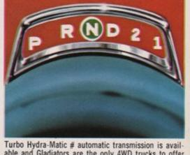
able and Gladiators are the only 4WD trucks to offer it! Here is fully automatic shifting through three forward speeds for easier going on or off the road. It's initial torque multiplication provides quicker acceleration than standard 3 or 4-speed transmissions.
