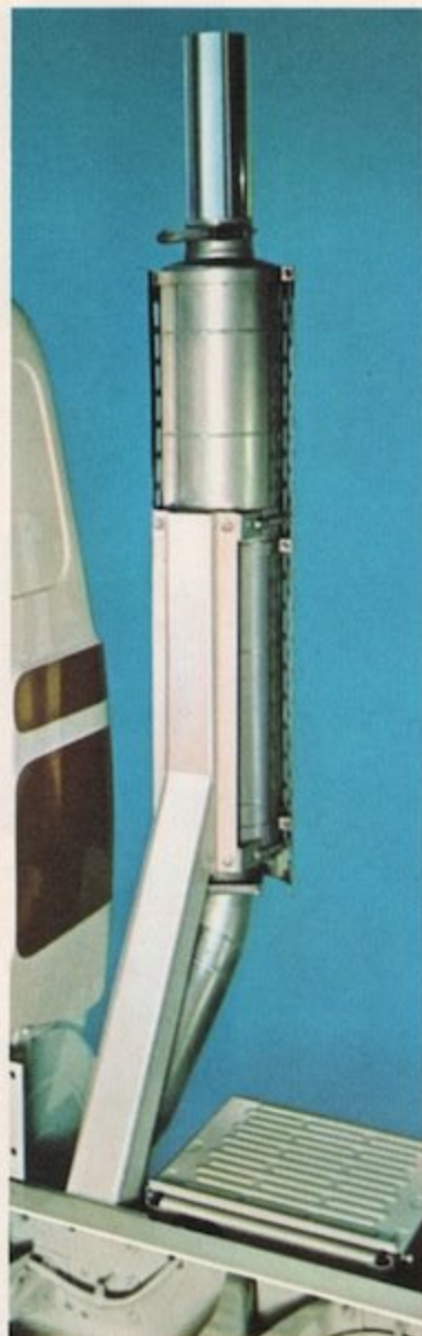
Freestanding exhaust stack, standard on some models and available on others, helps isolate road shock. Sturdy channel frame mount with side brace assures durability.
