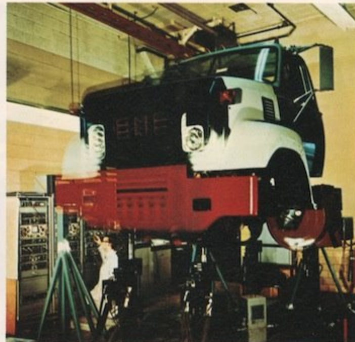
Torture Testing Delivers Quality . . . All GMC cab designs are expected to take a beating in any trucking application. Here a test unit undergoes a simulated round-the-world run encountering conditions that create the same type of shocks, stresses and sheet metal twisting found in the roughest operating situations. The split frame photo shows the cab at rest and under test. Because we apply tough standards in designing, testing and manufacturing, you get durability and serviceability from the Truck People from General Motors.
