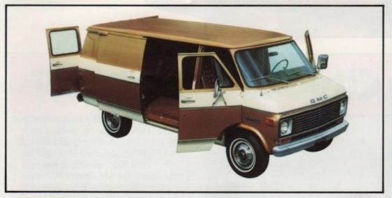
The Vandura's rear doors open nearly perpendicular to the sides of the van. That lets the driver back up close to loading platforms for easier and more convenient cargo loading. The side sliding door protrudes only 41/2 inches from the side of the van when fully opened-another plus for easy loading in cramped quarters. GMC Vandura knows you want to get the job done as soon as possible so you can get back to business.
