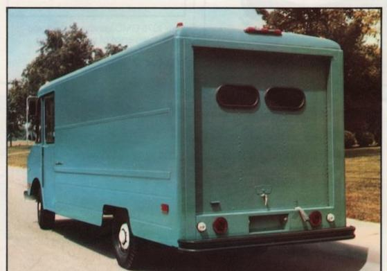
This body is ruggedly built inside and out to take on your toughest jobs. The steel body is strong and durable. On TP-208 model, overall length is 220¾" on a 125" wheelbase; side door openings are almost 32" wide, and the rear double doors open to 38" wide and almost 65½" high; storage area is 122" long. Depending on model, curb weights range from 4311 lbs. (TP-10) to 6242 lbs. (TP-314).
