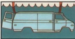
GMC helps protect every Vandura from rust and corrosion with the Elpo dip, which coats every surface of the van, including hard to reach crevices. You can be sure your Vandura will be working for you a long time.
