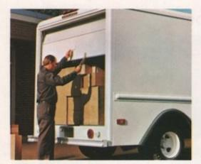
Available overhead rear door is counterbalanced and easy to handle; 66 inches wide on 10 foot narrow steel bodies, 78 inches wide on 10 and 12 foot steel bodies. Eighty-five inch doors are available on 10 and 12 foot aluminum bodies.
