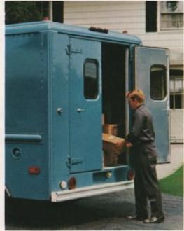
Standard rear doors are 38 inches wide and hung on full length piano type hinges on steel models and straptype hinges on aluminum models. 60 inch wide doors are available on all body sizes; 74 inch wide wraparound style on 10 foot steel bodies.
