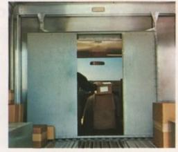
Available interior items include: sliding partition; auxiliary seat with seat belts; soft ray tinted glass, wood grained instrument panel, body height addition to 76 inches inside and all weather air conditioning for front (driver area).
