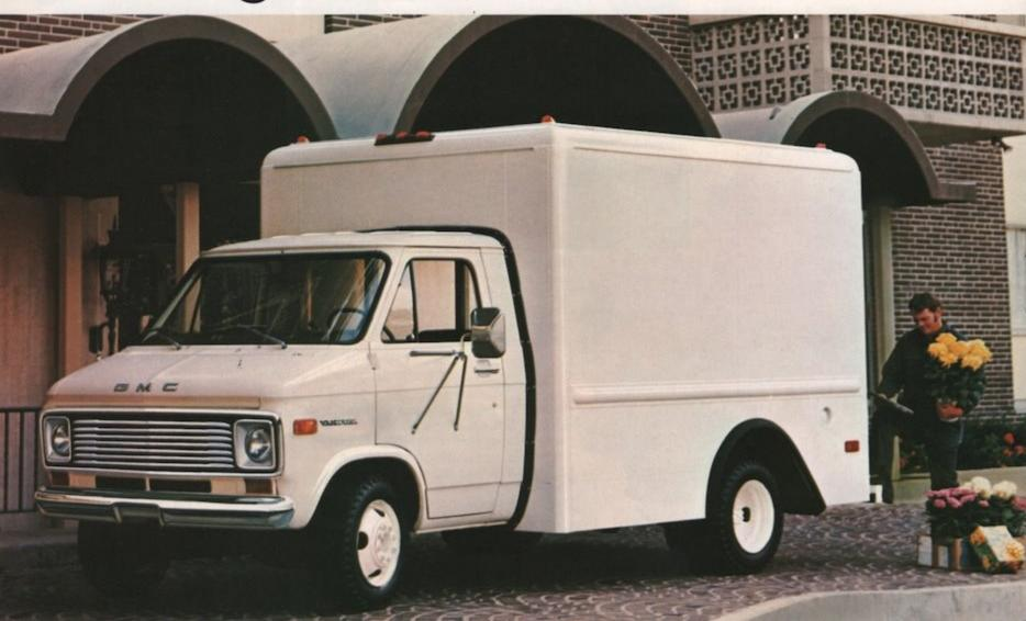
MagnaVans with available 82" wide 10 ft. steel body have a GVW range of 7400 to 8400 lbs. with the standard 292 In-line six engine and an 8,400 lb. GVW rating with a V8 engine; 8,900 lbs. with the 10 ft. aluminum body or the 10 ft. steel, 96 inch wide body. Twelve foot steel or aluminum bodies on the available 146 inch wheelbase models with dual rear wheels provide an 8,900 lb. GVW rating; 10,000 lb. GVW units available with 7,500 lb. rated rear axle.
