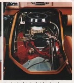
Engine maintenance is easy with Vandura's standard extended front end design. You can do a fast 27-point check on normal service items. Water fill, oil fill and check, battery, windshield washer fluid reservoir and brake master cylinder are at your finger tips. The insulated engine compartment cover inside the vehicle is removed quickly allowing for other routine engine service work.
