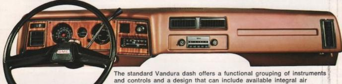
The standard Vandura dash offers a functional grouping of instruments and controls and a design that can include available integral air conditioning with facing directional vents. Non-reflective surfaces reduce glare; soft control knobs are marked with international symbols for easy identification. Voltmeter, oil pressure and water temperature gauges are available as a package.
