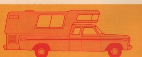
SLIDE-IN CAMPERS. Slide-in campers can change your pickup from truck or second car to camper in a matter of minutes. Generally, slide-ins have a cab-over section that contains the main sleeping area. Slide-in campers range from 6 to 11 feet in length and cost from about \$1000 to over \$5000.
