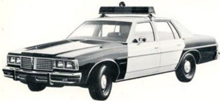
4-Door Sedan and 4-Door Wagon Wheelbase 115.9" (2 944 mm)
