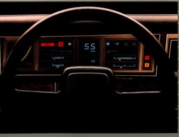
latest in high-tech instrumentation. The **Electronic Cluster** features digital readouts for speedometer, odometer and electronic gauges for oil pressure, fuel, coolant temperature and electrical voltage.
