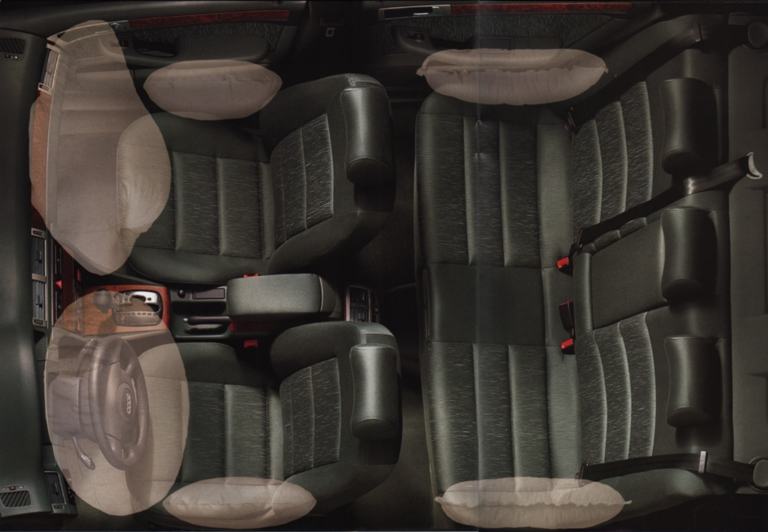
Four airbag supplemental restraints in the front are standard on the A8. With the Enhanced security package, the option of two more in the rear.
