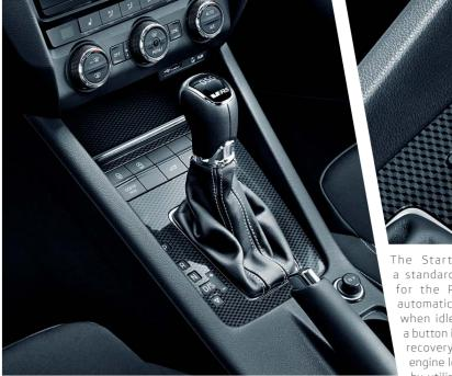
While the front-wheel drive is combined with an automatic 6-speed battery recharging. DSG (Direct Shift Gearbox) or a manual 6-speed transmission, the 4x4 drive is always accompanied by an automatic 6-speed DSG.
