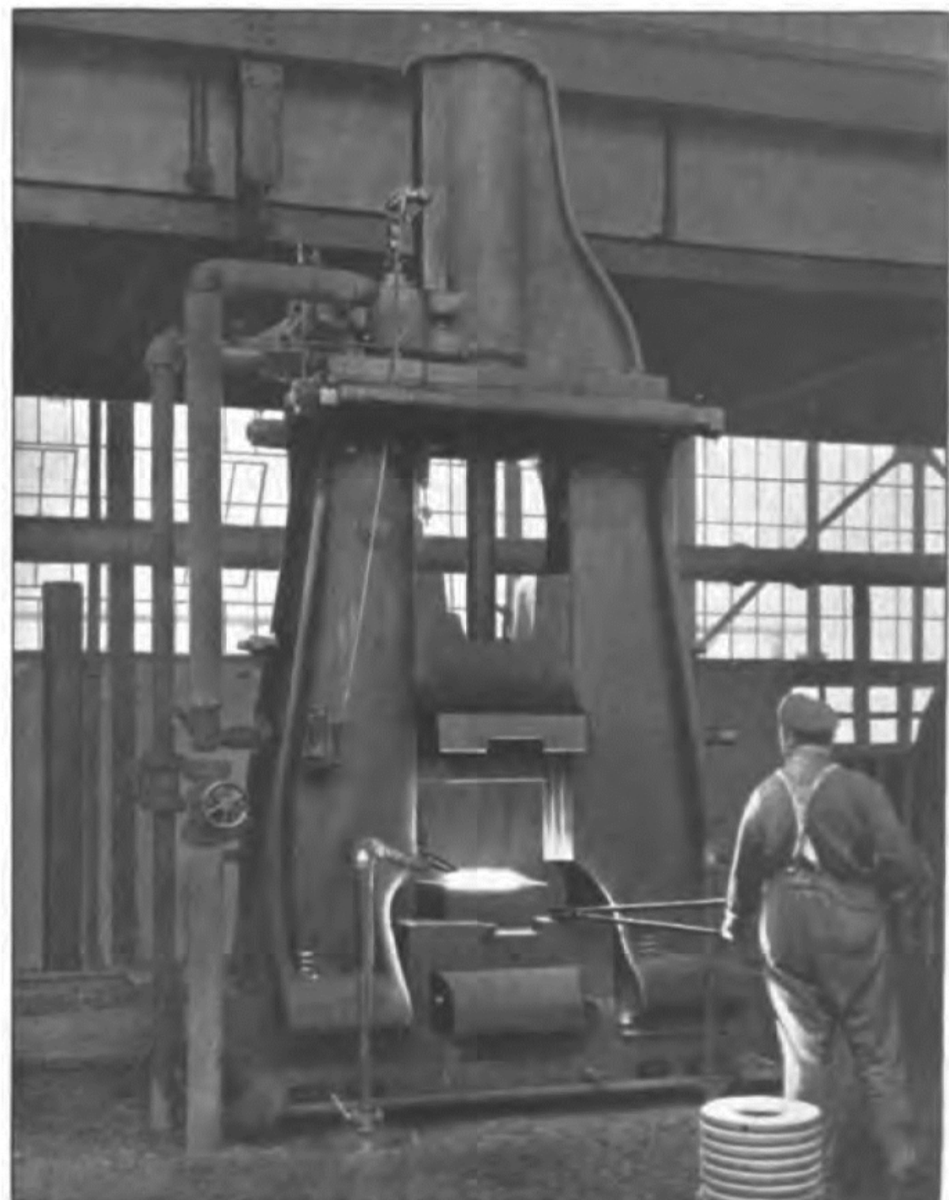
A GEAR BLANK GOING UNDER THE HAMMER IN THE PACKARD FORGE
