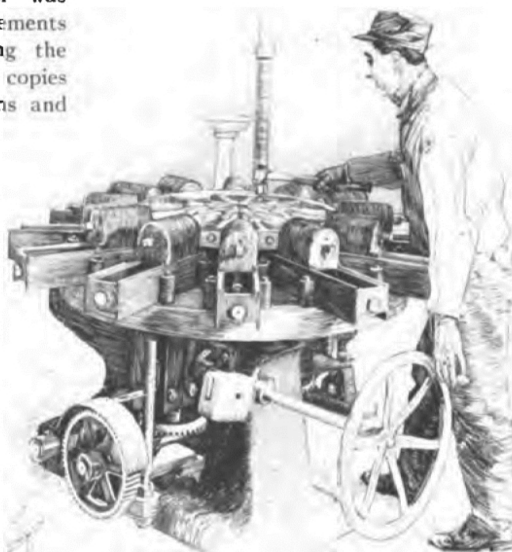
THE SQUEEZING POWER OF THIS MACHINE IS ABOUT FOURTEEN TONS
