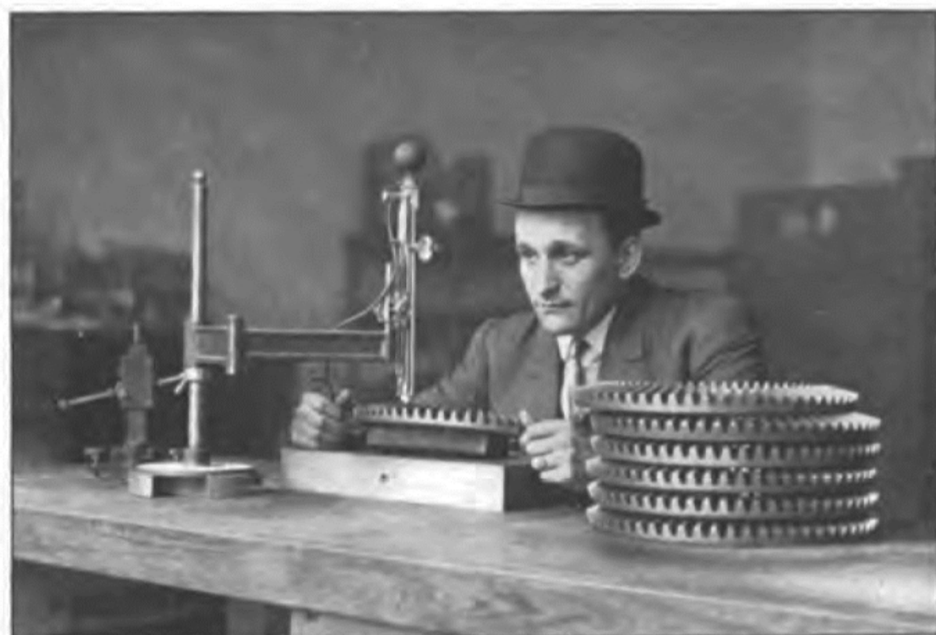
JOE BRODIE USING THE SCLEROSCOPE IN TESTING A GEAR FOR HARDNESS
