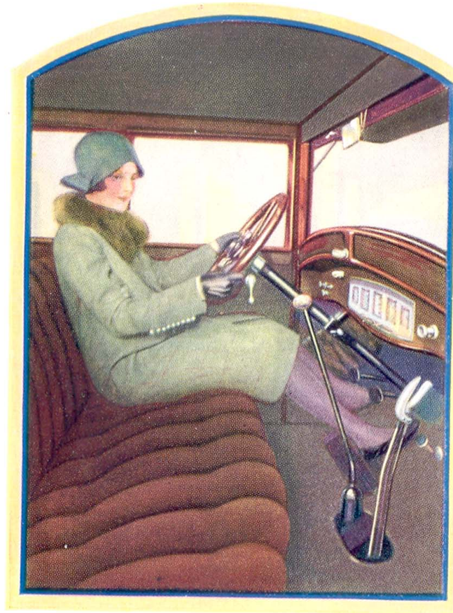
(ABOVE) Convenience characterizes every detail of the President's design. Before your eyes are: gasoline gauge, speedometer, engine thermometer, eight-day clock and other indicators, all set under glass and indirectly lighted. The coincidental steering-ignition lock has a special light. Twin-beam driving lights and cowl lights are controlled from steering wheel. No-draft ventilating windshield adjusted from the dash. Horn button and shift lever ball are onyx. A cigar lighter is mounted at right of instrument panel.
