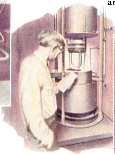
This "fadeometer" duplicates the effect of extreme heat and cold, the sun's ultra-violet rays and rain on lacquers, top material and upholstery used in Studebaker cars.
