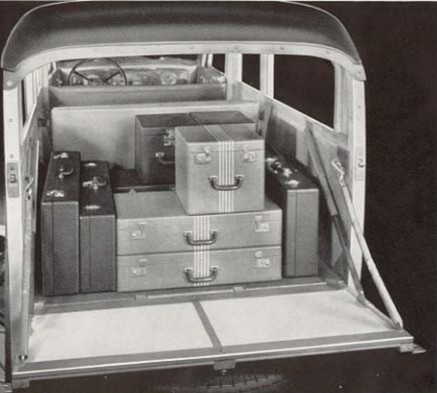
The 2-passenger seat is easily removed and the 3-passenger seat simply moved forward to leave additional baggage room at the rear. There are 12 pieces of luggage illustrated in place here and space for more, even with the tailgate snapped shut. No seat or floor bolts project, to mar or scratch.
