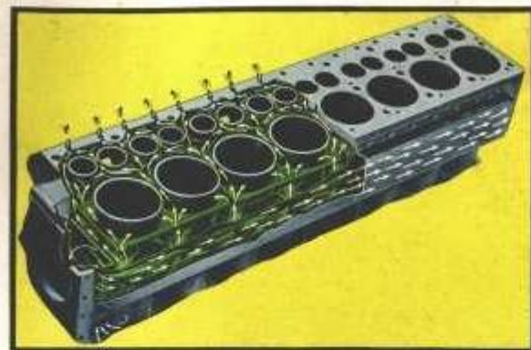
A study in "busy" water—its flow directed for uniform cooling, penetrating to all points where power-stealing heat must be removed.
