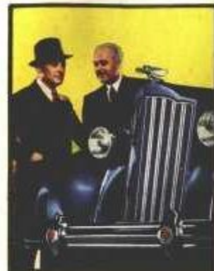
No mere ornamental grille here—but chrome shutters that are both handsome and useful. The automatic vanes control temperature for maximum power.
