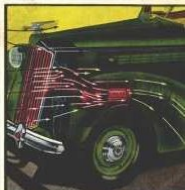
Packard—and Packard exclusively—provides these fan blast cooling tunnels for removal of heated air.
