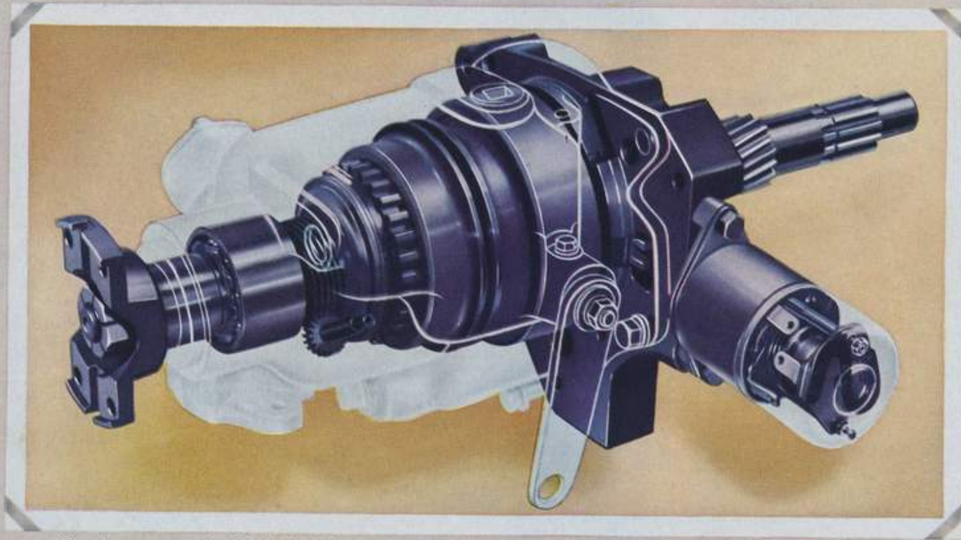
Here, in a compact, simplified unit, is the improved 1940 Packard Econo-Drive—an investment in pleasure and economy worth far more than its moderate extra cost. At speeds as low as 21 miles per hour, this thrifty fourth speed reduces engine speeds by 27.8%—saving on gasoline, oil and engine wear. Performance becomes incredibly smooth and quiet.
