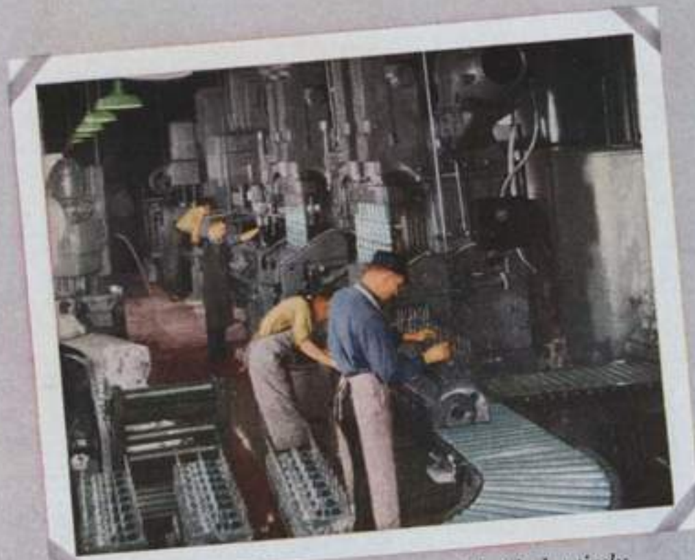
Packard engine blocks are cast and finished entirely under the Packard roof. This honing machine imparts a mirror-like finish to cylinder wall surfaces.
