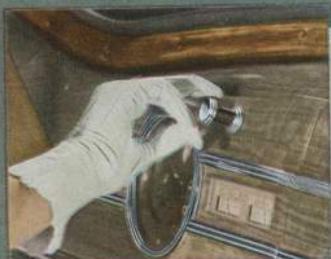
Dash illumination—for ignition key or dials—is easily adjusted to any degree of brightness by a handy rheostat.
