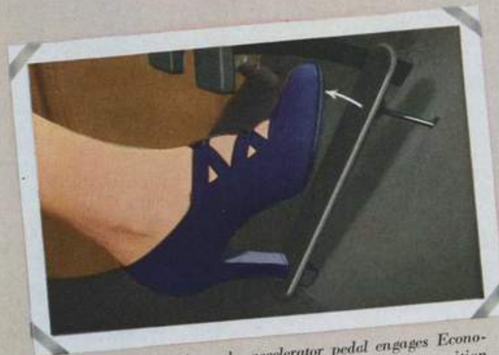
Here, in a compact, simplified unit, is the improved 1940 Packard Econo-Drive—an investment in pleasure and economy worth far more than its moderate extra cost. At speeds as low as 21 miles per hour, this thrifty fourth speed reduces engine speeds by 27.8%—saving on gasoline, oil and engine wear. Performance becomes incredibly smooth and quiet.
