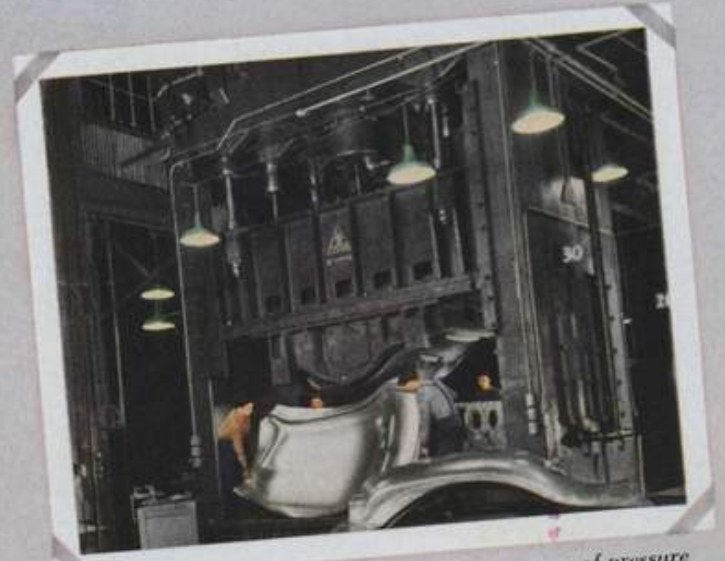
Giant presses more than two stories high exert tons of pressure as they stamp bodies out of solid steel sheets. Even the largest shapes are pressed in Packard's own mammoth stamping mill.
