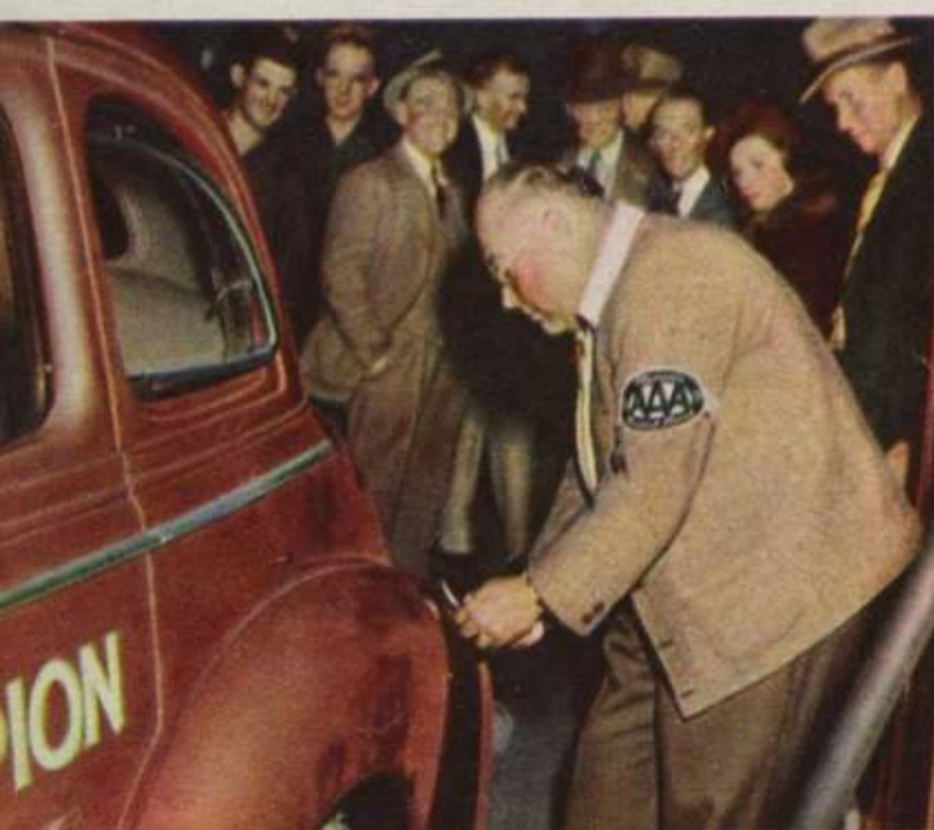
Gas tank is sealed by A.A.A. official—and the seal will be broken only by an official A.A.A. observer traveling with the car. Every drop of gasoline and oil used by this stock model Champion will be impartially measured and checked.
