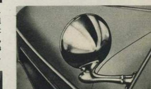
Controllable spotlight may be focused in any desired direction from the car interior. Locates signs and numbers easily.
