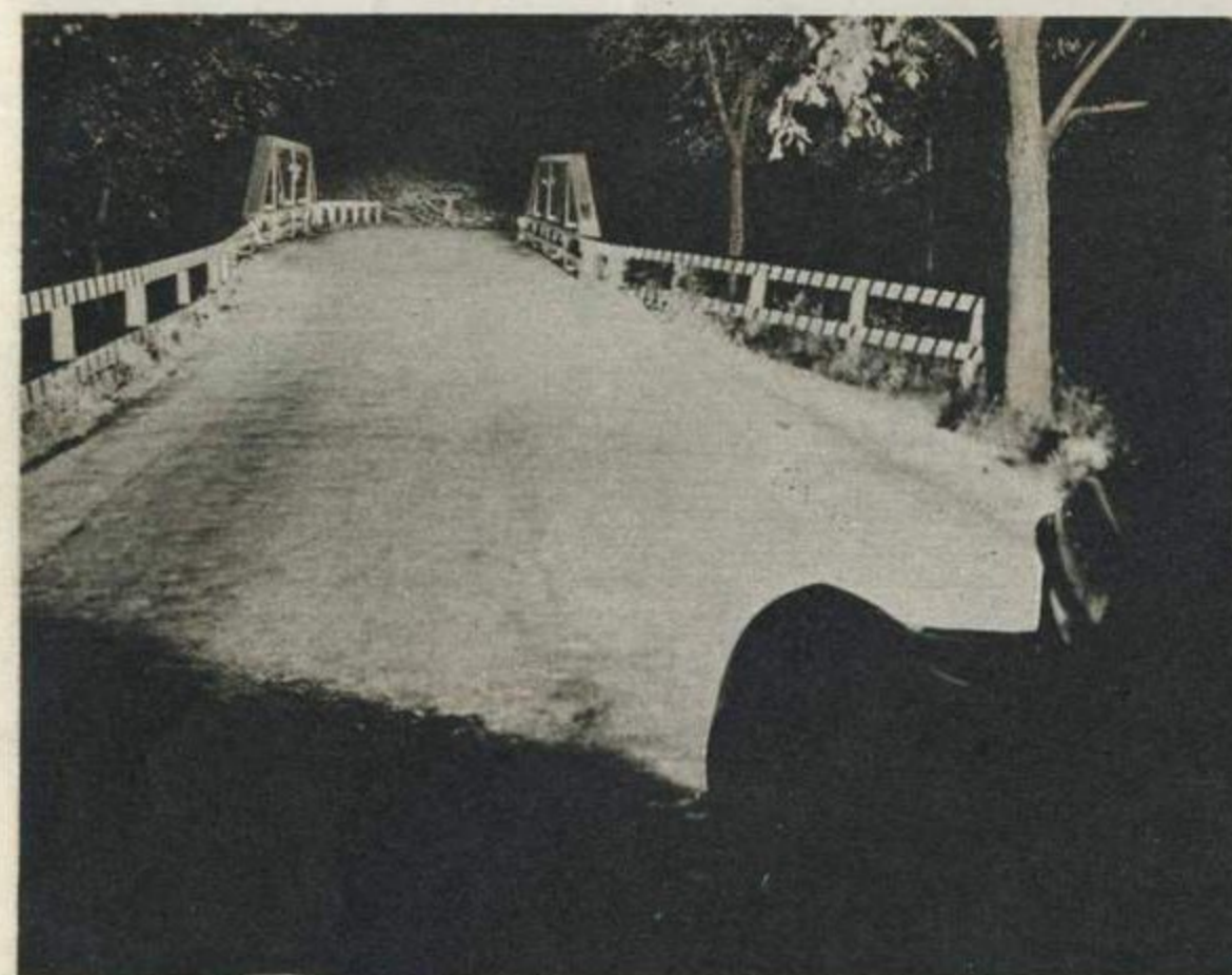
Here's how the Studebaker Champion's "sealed beam" headlamps light up the whole road—This advanced lighting method takes its place as a safety factor alongside four wheel brakes and safety glass. It makes night driving simpler and less of a strain because of the more efficient illumination and the permanently fixed focus of the two headlamp beams. A toe switch deflects the light for passing oncoming cars.
