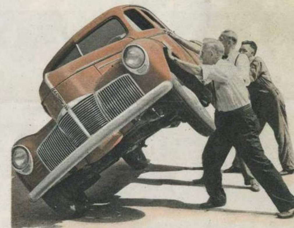
They're showing how beautifully balanced this 1940 Studebaker Champion is—You can tilt a Champion to an angle of more than 57½ degrees without danger of upsetting it. That's because of the Champion's unusually low center of gravity which enables it to hug the road even when rounding turns at cruising speeds.
