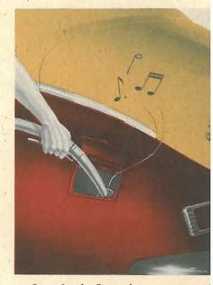
Gas Tank Signal speeds filling, ends spillage. When its whistle stops, tank is filled to proper level with allowance for gas expansion.
