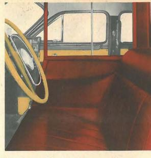
Convenient reading light is at your shoulder. Radio and underseat heater are popular extras. Note, too, the special footrail for front seat passengers, and the safety pad on instrument board.
