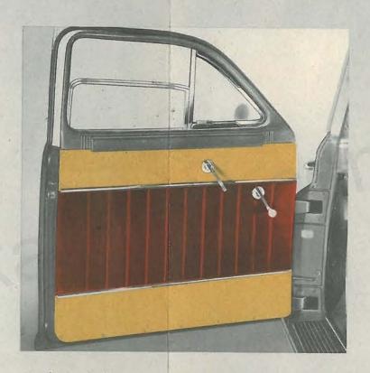
Upheep Cutters—these are typical: Windows have metal frames; door latch is special for heavy-duty cab work; door check is husky—but if broken can be replaced in about 10 minutes, without welding. Doors have no-slam rotary latches.
