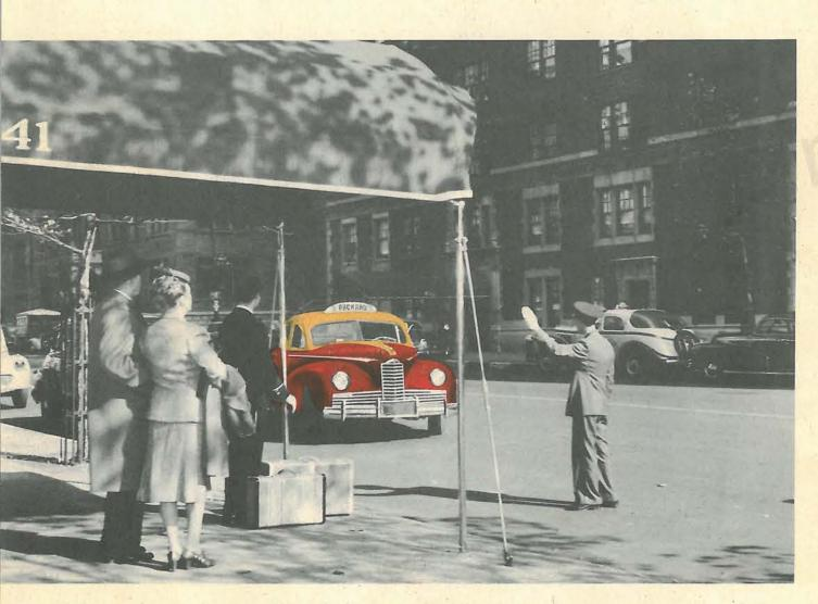
2uich Turning, Easy Parking. Wheelbase of the new Clipper Cab is 120 inches, turning radius only 21 feet. Parking is easy—and there's a back-up buzzer
