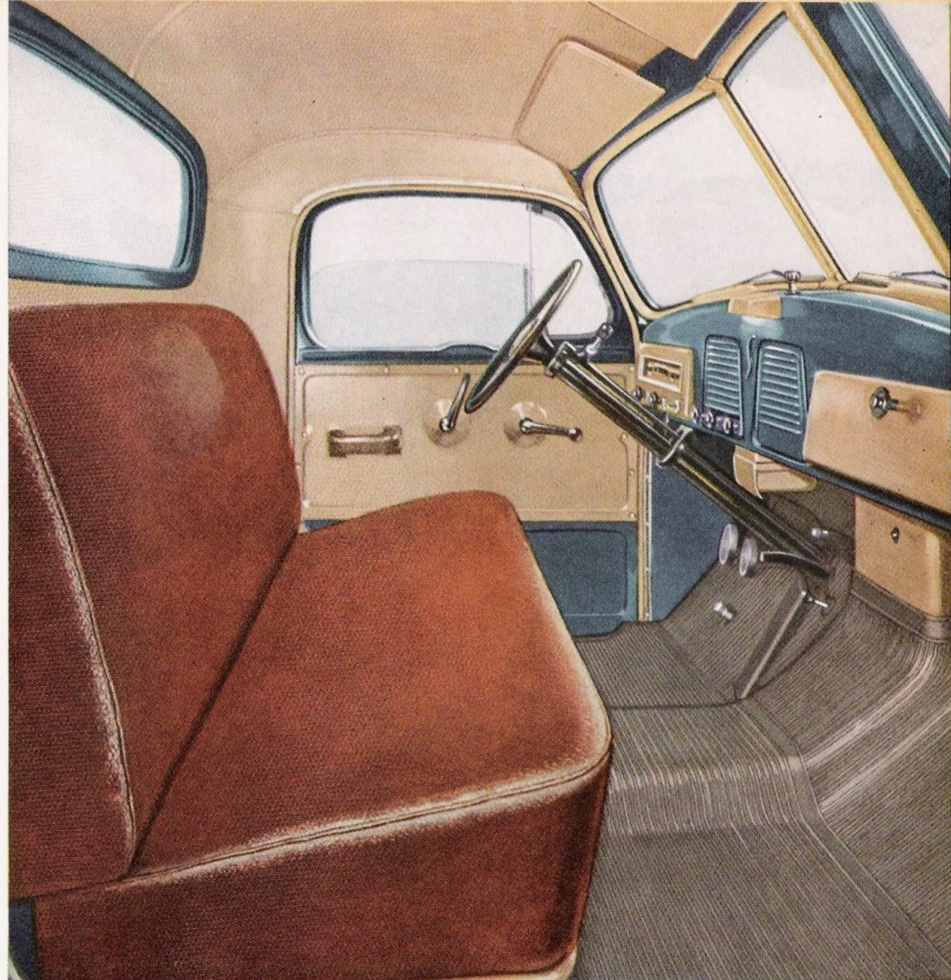
Steering post gear shift standard on 1/2-ton and 3/4-ton models with 3-speed transmission or overdrive.
