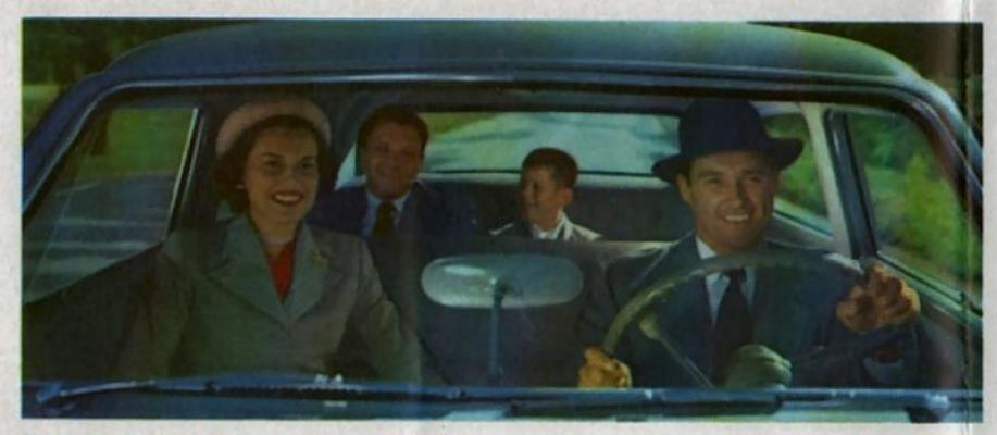
Tinted "green" glass available in windshield and all windows is Studebaker's newest contribution to comfortable motoring. Eye-fatigue, due to glare from brilliant sunlight or strong night lights, is reduced. This glass helps to temper heat from summer sun. Available on all models at extra cost.
