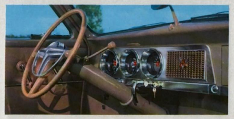
The Commander instrument panel has big, sweep-type aircraft dials. The electric clock is standard on Land Cruiser and available on other models at extra cost. Smart, sure-grip steering wheels. Pistol-grip parking brake handle. Large package compartment with easy-to-open lock.
