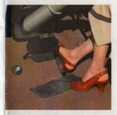
No clutch pedal! The brake pedal is oversize, gives added safety and may be used with either foot. You can't start the engine when car is in gear.
