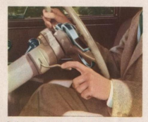
Built-in directional signal equipment is available as an extra cost accessory. Gives added safety. Front and rear lamps flash intermittently on either left or right hand turns.
