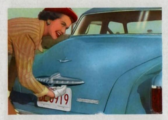
An easy-acting weather-protected trunk lock is built into the trunk lid handle on all models. Spherical-type handle on Custom Champion. The counterbal-anced trunk lid opens and closes with finger-tip ease.
