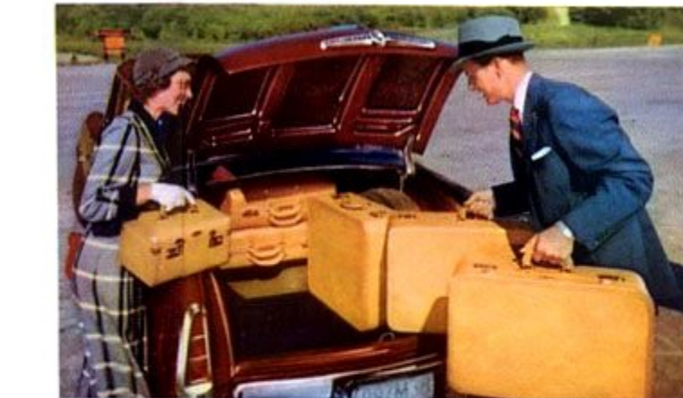
Plenty of room for all the family luggage in this spacious sedan trunk. A "wing" type trunk lock release makes it easy to open the trunk. Thanks to "over-the-center" springs, the lid requires very little effort to lift.
