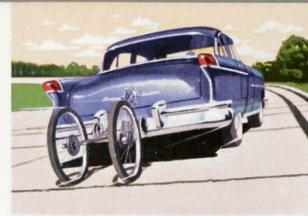
THE INSTRUMENTS mounted on the "bicycle wheel" carriage measure speed and acceleration with utmost accuracy on the world's fastest 2½-mile closed track.
