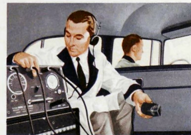
HERE IS how distracting noise is ferreted out and its origin determined. This instrument scientifically records the sound-level in every section of the car's interior.
