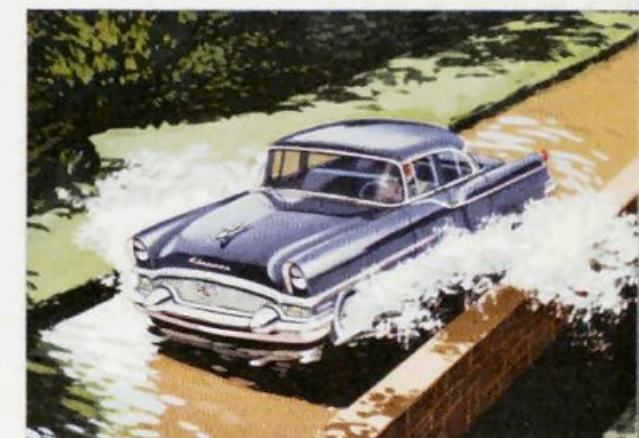
SENDING twin sprays flying, a Clipper sweeps through the water bath. This thoroughly tests chassis, engine and electrical system for waterproof qualities.
