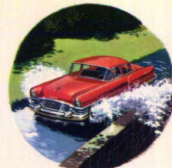
Moisture-proof ignition and waterproof bodies are repeatedly checked by Packard Engineers in this water bath. Cars are driven at various speeds through varying depths of water to insure Packard performance under all conditions.
