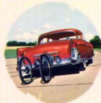
Gasoline mileage, acceleration, braking and maximum speed are tested on the world's fastest 2½-mile track at the Packard Proving Grounds. Bicycle wheel instrument provides perfect calibration and recording of accurate tests.
