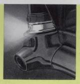
All Packards and Clippers are equipped with backup lights. A broad beam of white light is directed behind the car to provide maximum backing visibility and alert other drivers and pedestrians that you are in reverse. Backup lights are automatically operated by a switch on the Ultramatic selector linkage or on standard transmissions by contact when the lever is placed in Reverse.
