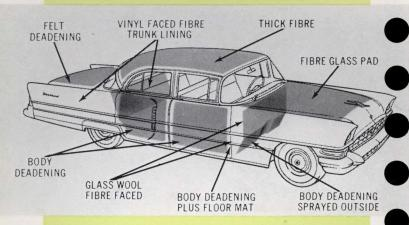
High quality insulating materials are used throughout Packard and Clipper cars to increase passenger comfort by controlling noise or temperature changes.
