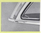
Packard and Clipper door handles are rigidly mounted at the car's belt moulding. Handles are positioned at the correct door opening height and also enhance the smooth clean body line. The door handles are all push button operated for convenience and easy operation.
