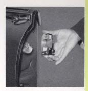
On all Packards and Clippers an interlocking striker plate overlaps the door latch rotor. This feature prevents the door from flying open in a sudden impact. This keeps passengers within the car, reduces chance of injury.
