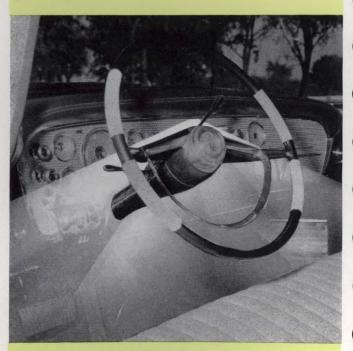
Center front courtesy light, located under the center of the Packard and Clipper instrument panel, is operated automatically by either front door. Effectively illuminating door openings and car floor, it also serves as a map light when operated by the headlight switch.
