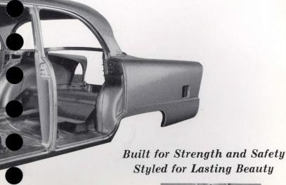
Sturdy box-section center pillars are flared in three sections. The front and rear flared sections are welded to the floor panel. The inside section is welded and bolted to the car frame.
