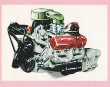
Packard V-8 Power gives the Station Wagon instant acceleration, smooth cruising pace and safe reserve for passing in traffic or on long upgrades. The 289 cubic inch engine develops 225 horsepower, is of advanced short-stroke design, and has automatic controls for sustained efficiency.
