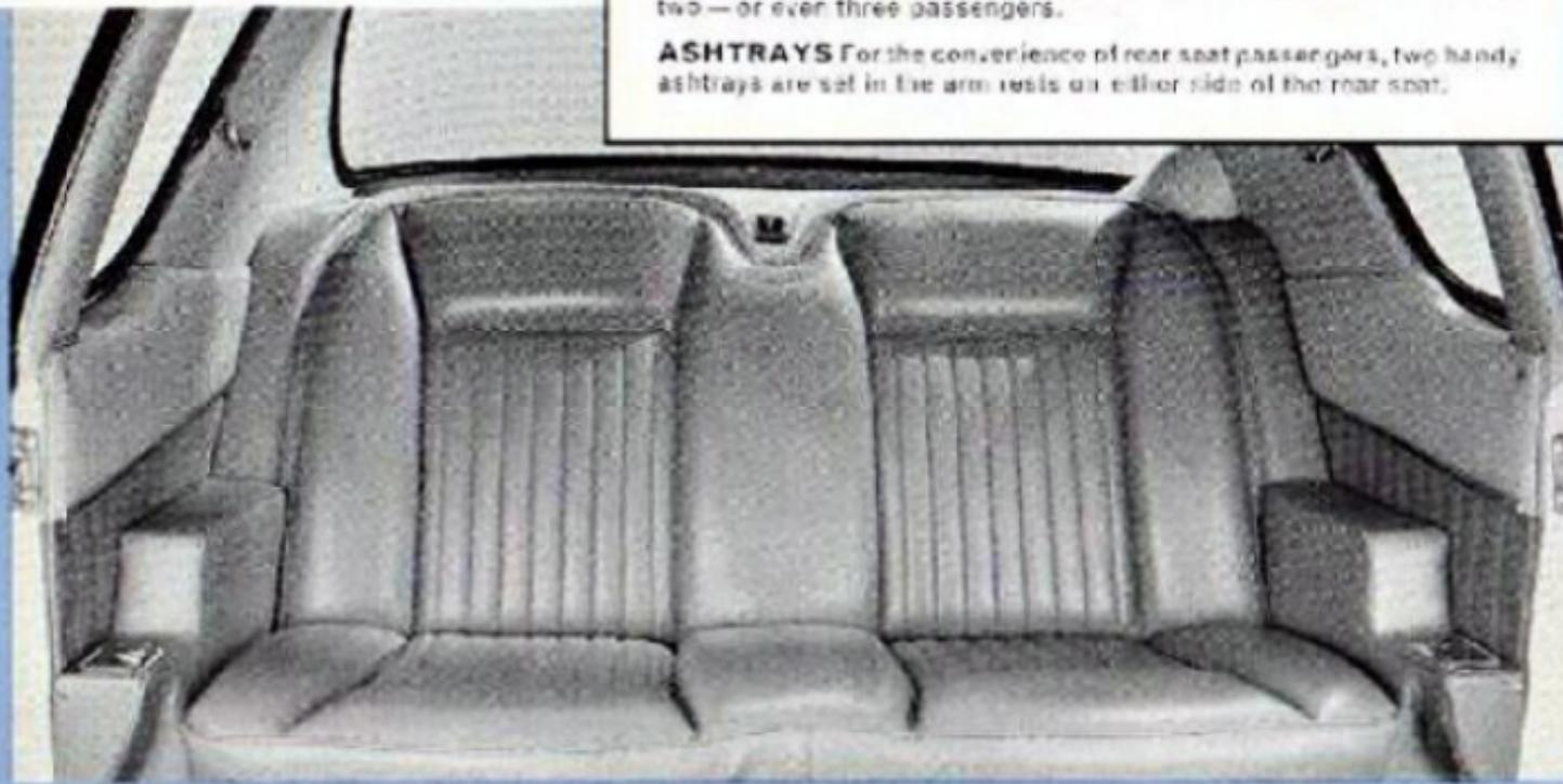
**CONTOURED REAR SEAT** There's plenty of legroom, headroom and hiproom, too, in the slightly elevated rear passenger compartment. The seat is body contoured to afford the utmost in lounge-chair comfort. Soft, pliable foam-rubber is used to cover the base of the comfortable seat. Deep coil springs are used in rear seat construction. The rear seat is also covered in attractive, washable Textileather. There's room for two—or even three passengers.
