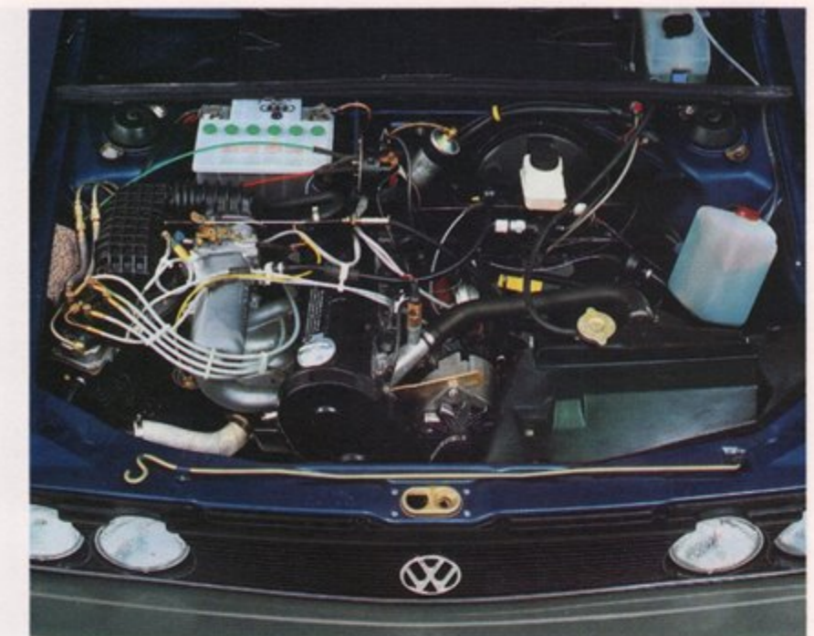
FUEL INJECTED, 1.6 LITER OVERHEAD CAM ENGINE.
