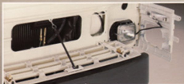
New grille design improves air flow and engine cooling. Integrated turn signals are better protected and offer improved aerodynamics.
