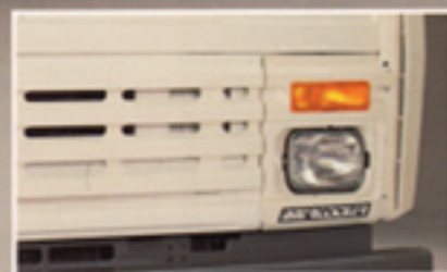
New grille design improves air flow and engine cooling. Integrated turn signals are better protected and offer improved aerodynamics.
