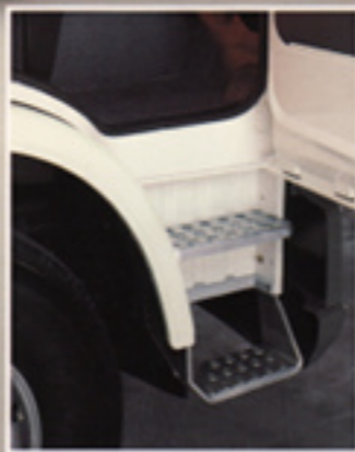
Two serrated, self-cleaning steps provide surer footing to make cab entry/exit easier and safer.
