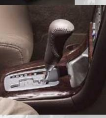
A 4-speed electronically controlled automatic transmission is standard in all Outback H6-3.0 models. The gated shifter provides precise control for manual gear shifting, if desired.
