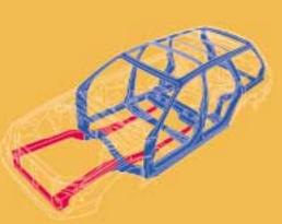
Ring-Shaped Reinforcement Frame construction is one reason that Outback models offer outstanding safety. This design ties together structural elements in the floor, sides and roof to form a strong steel cage that helps protect the passenger compartment should an accident occur.
