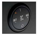
**POWER TAKEOFF (PTO) CAPABILITY**<sup>1</sup> allows HD Chassis Cab equipped with this GM segmentexclusive feature and the available Allison 1000 Series six-speed automatic transmission to power auxiliary equipment such as a dump body or hydraulic motors for generators or tools.
