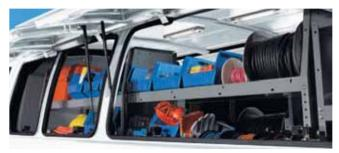
**AVAILABLE ACCESS PACKAGES** offer easy interior access to tools and cargo. Each includes three exterior, remote-release, side-access panels that can be opened by Remote Keyless Entry. Not available with optional driverside 60/40 swing-out doors or sliding passenger-side door.
