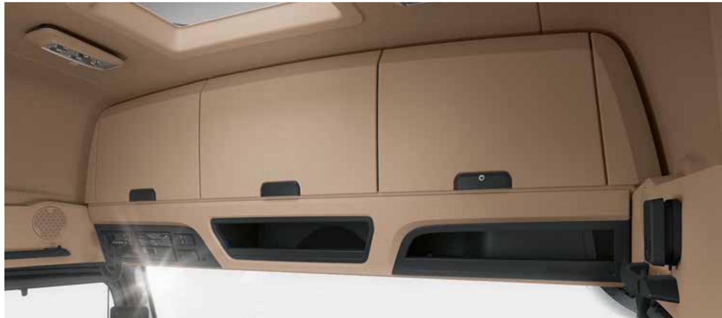
**Stowage compartments above the windscreen.** As a result of the new, symmetrical arrangement of the stowage compartments above the windscreen, the GigaSpace offers not only 332 l of stowage capacity, but also excellent freedom of movement and headroom on the co-driver's side. The upper stowage compartments with hinged lids are illuminated on the inside, lined with slip-resistant felt and offer two drivers adequate space for everything they need to take along with them.
