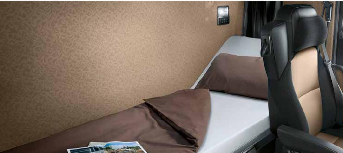
**Maximum comfort for resting and sleeping.** With upper and lower beds each measuring 750 mm in width and up to 2200 mm in length<sup>1)</sup>.
