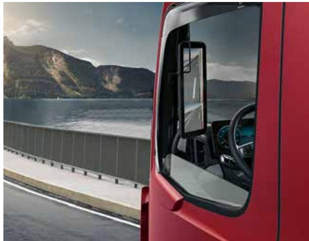
**Side window wind deflector.** The aerodynamically optimised tinted or clear side window deflector set for the driver's or co-driver's side protects against the airflow when driving with the windows open.
